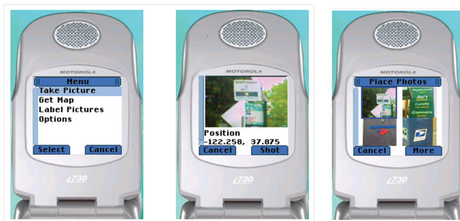
Figure 5.7: Cell phone interfaces for Photo . (number order - left to right) 5.7.1 is the initial interface after activation. 5.7.2 is the photo capture interface. 5.7.3 is the photo history. After pressing the ok button in 5.7.3, the DText interface will pop up.
