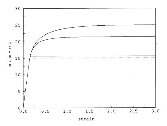
Figure 1: Uniaxial tension test: rate dependent effects. Dependence on the characteristic time: stress versus strain.
