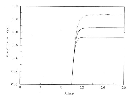
Figure 7: Thin walled tube in tension and torsion. Tangential stress  $\sigma_{z\theta}$  versus time.
