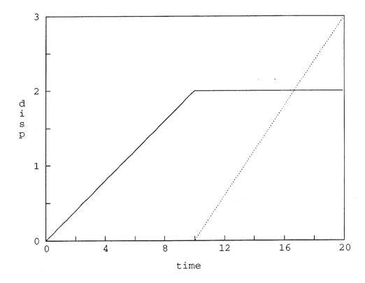
Figure 5: Thin walled tube in tension and torsion. Time history: normal and tangential displacements versus time. The tangential displacement is reported with a dotted line.
