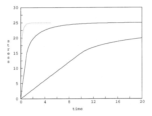
Figure 2: Uniaxial tension test: rate dependent effects. Dependence on the loading rate: stress versus time.
