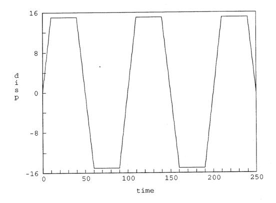
Figure 3: Uniaxial tension test: cyclic loading. Time history: displacement versus time.
