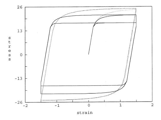
Figure 4: Uniaxial tension test: cyclic loading. Stress versus time.  $\sigma_y = 15$ ,  $\beta = 10$ ,  $\delta = 20$ ,  $H_{iso} = H_{kin} = 0$ . Loading rate p = 1 = const, characteristic time  $\tau \in \{0.1, 1, 10\}$ . The solution for  $\tau = 10$  is reported with a dotted line.
