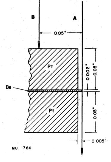
An electron following the orbit A (with its center to the left) passes through the beryllium fin, losing 15 Kev of energy; on the next time around it follows the path B, passing through the thick target. Dimensions correspond to the case given in the text, with H = 3 kilogauss, n = 3/4. An electron passing through the platinum target shown loses about 7 Mev by ionization.
