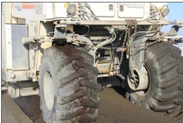
Figure 3.16: FDR-EE: Excess emulsion applied during recycling.
