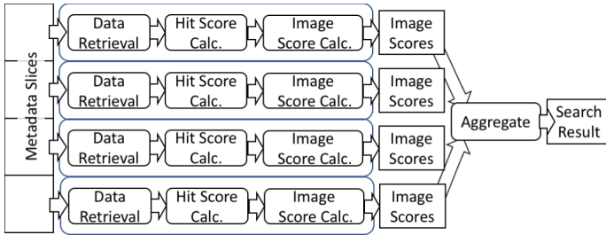
Fig. 10: Search metadata is sliced and processed by n workers that retrieve data, calculate hit scores, and image scores. Intermediate scores are aggregated to produce search results.
