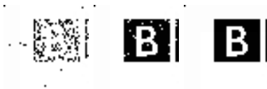
Figure 1.4. Stealing a 48 \times 48 pixel region from www.bbc.com , at 100 \times 100 , 200 \times 200 , and 300 \times 300 pixel-inspection div size.
