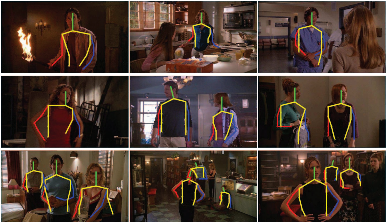
Fig. 13. Results on the Buffy dataset. We visualize all skeletons (instead of boxes) reported by our algorithm for a given image, after NMS. Our model hence serves as both an articulated detector and pose estimation algorithm, as evidenced by our APK measure.
