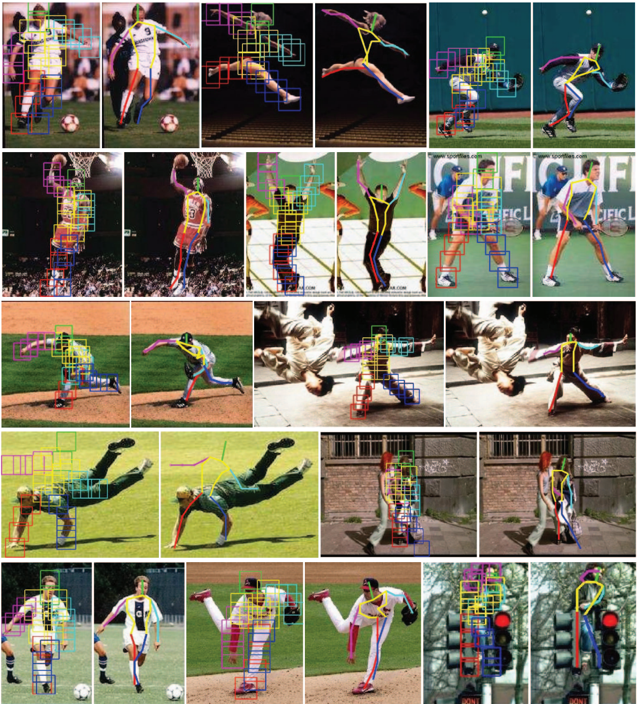
Fig. 12. Results on the Parse dataset. We show 26 part bounding boxes reported by our algorithm along with skeletons computed from the bounding boxes for each image. The top 3 rows show successful examples, while the bottom 2 rows show failure cases. Examining failure cases from top left to bottom right, we find that our model is not flexible enough to model horizontal people, is confused by overlapping people, suffers from the double-counting phenomena common to tree models (both the left and right legs fire on the same image region), and is confused when objects partially occlude people.
