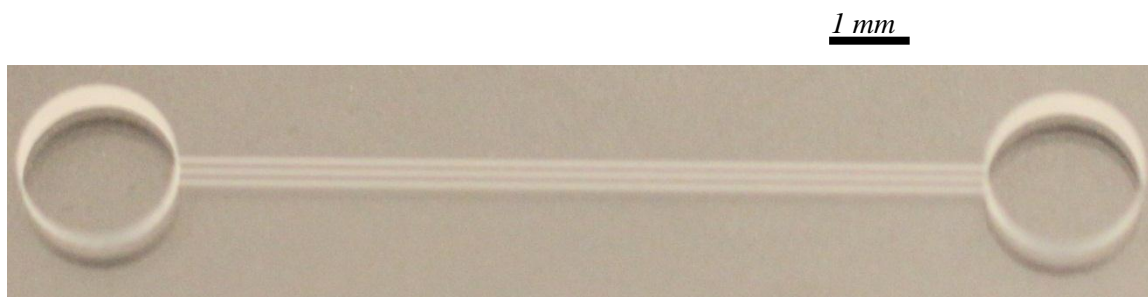
Figure 7.1: A glass chip housing three parallel microchannels forms the basic architecture for gel-based IEF immunoassay.
