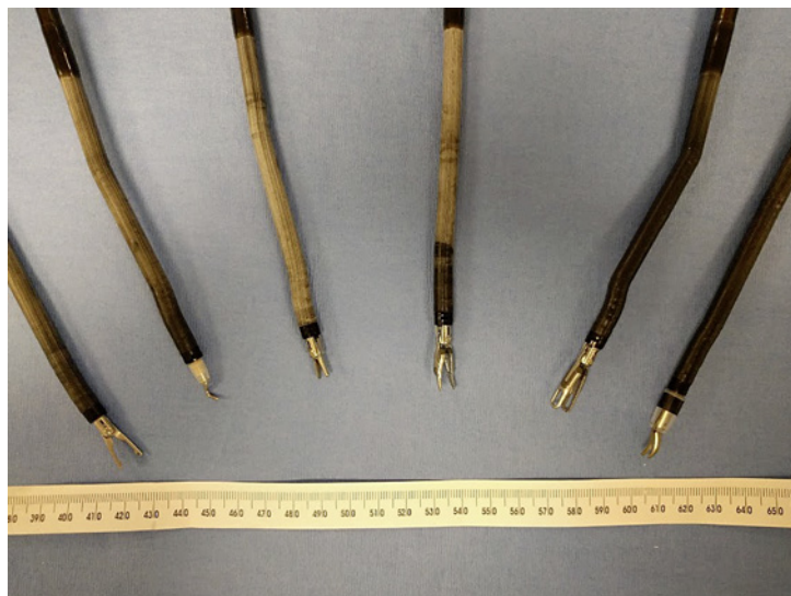
Fig. 4. da Vinci® Sp instrumentation. A variety of instruments will be available for the da Vinci® Sp system including energy devices (bipolar and monopolar instruments), needle drivers, grasping instruments, and clip appliers.
