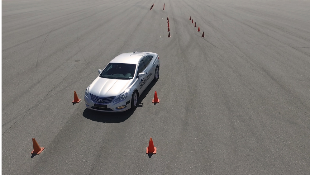
Figure 7.3: Experimental setup consisting of cones and the test vehicle entering the final segment of the test course
