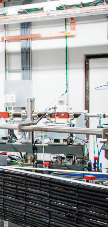
Achromats in the 1.5 GeV ring with the front end of the beamline SPECIES in the foreground. Photo: Madeleine Schoug.
