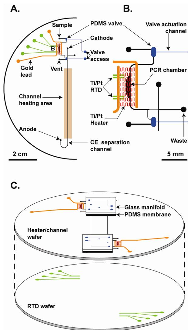
**Figure 3.1.** The design and structure of the microdevice.
