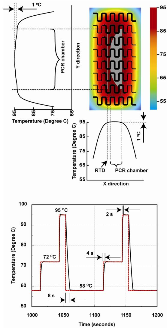
**Figure 3.2.** The design of the microfabricated PCR heater.
