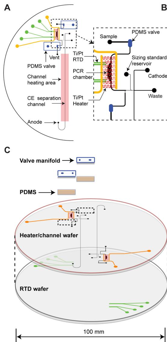
**Figure 4.1.** The design of the microdevice.
