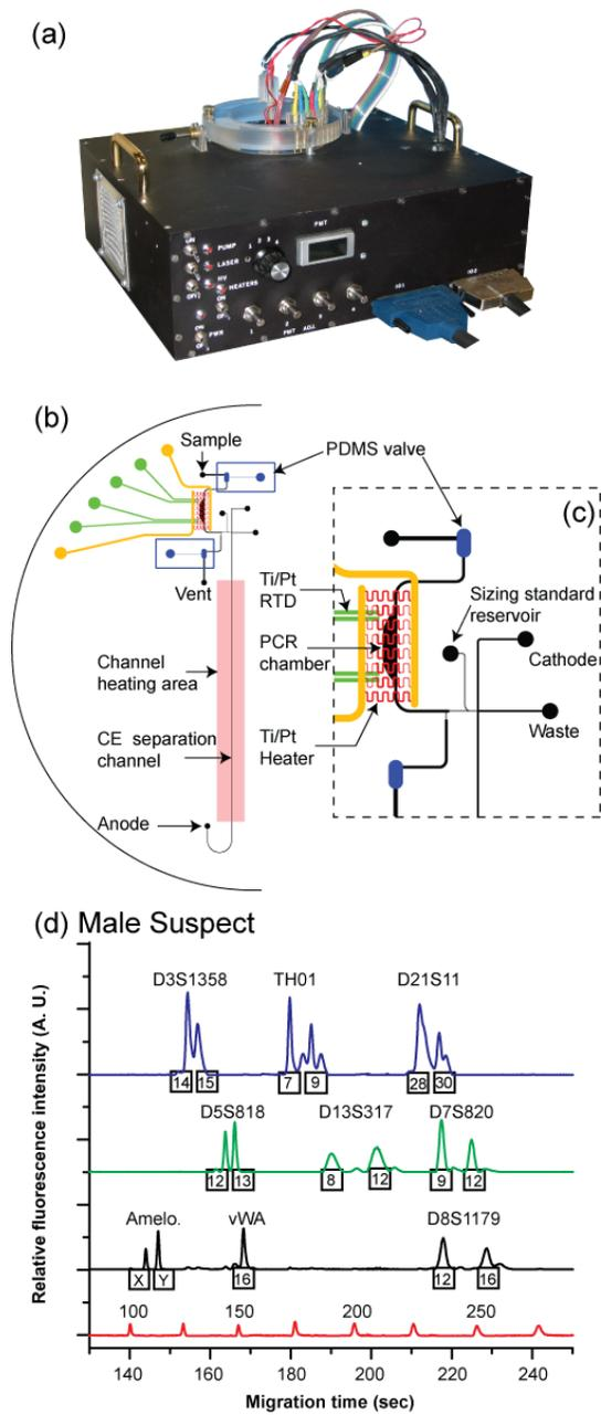
**Figure 2.5.** A portable integrated genetic analyzer for on-site forensic STR typing.
