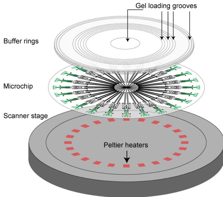
**Figure 6.2.** The exploded view of the microchip assembly.
