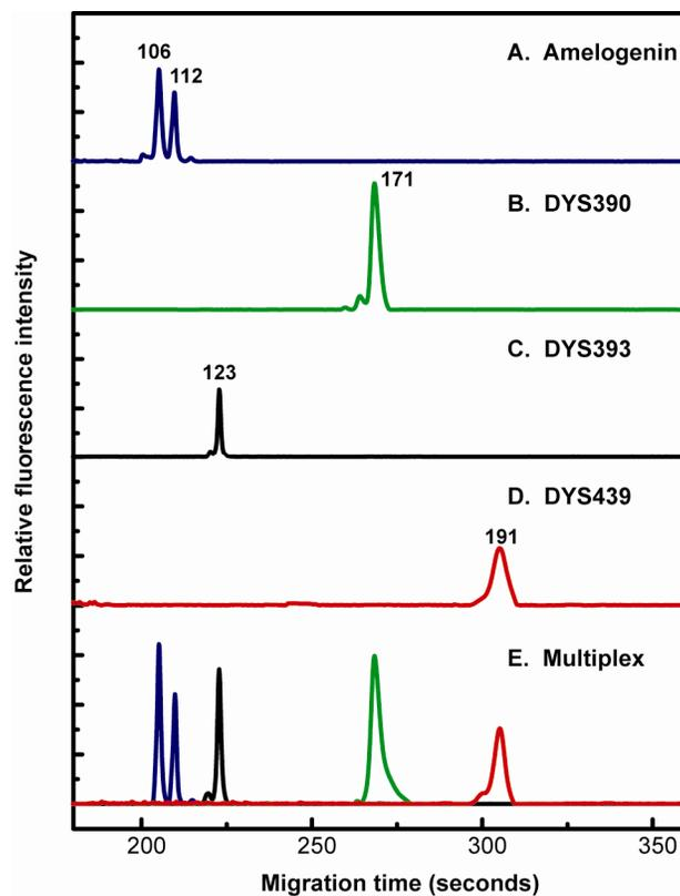
**Figure 3.4.** Singleplex and multiplex STR amplification performed on the PCR-CE microsystem.
