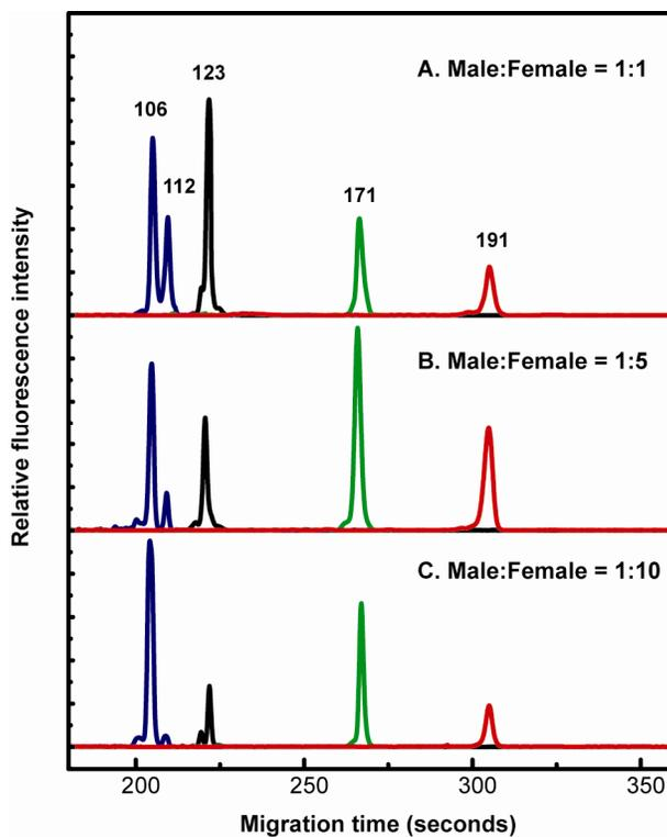
**Figure 3.7.** Mixture sample analysis using the PCR-CE microdevice.
