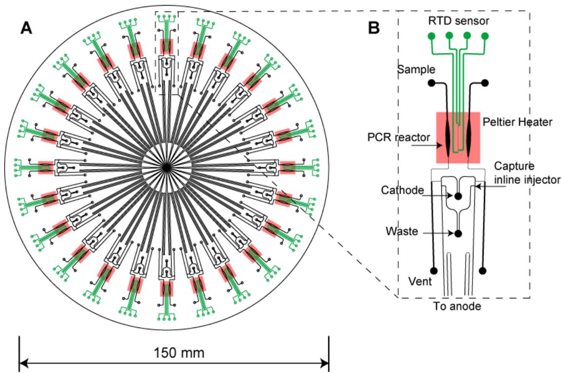
**Figure 6.1.** Schematic of the 48-lane PCR-capture-CE microdevice for forensic DNA Typing.
