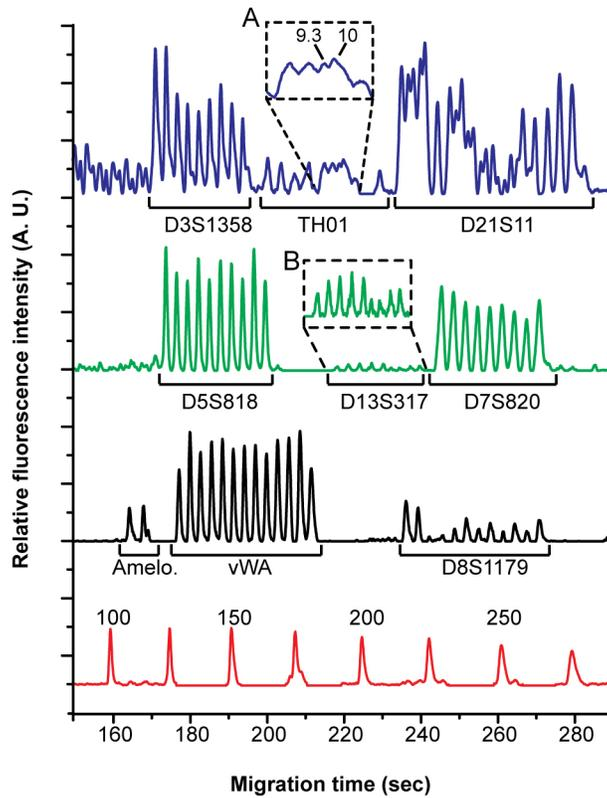
**Figure 4.3.** The 9-plex STR allelic ladder separation obtained on the portable PCR-CE microsystem.
