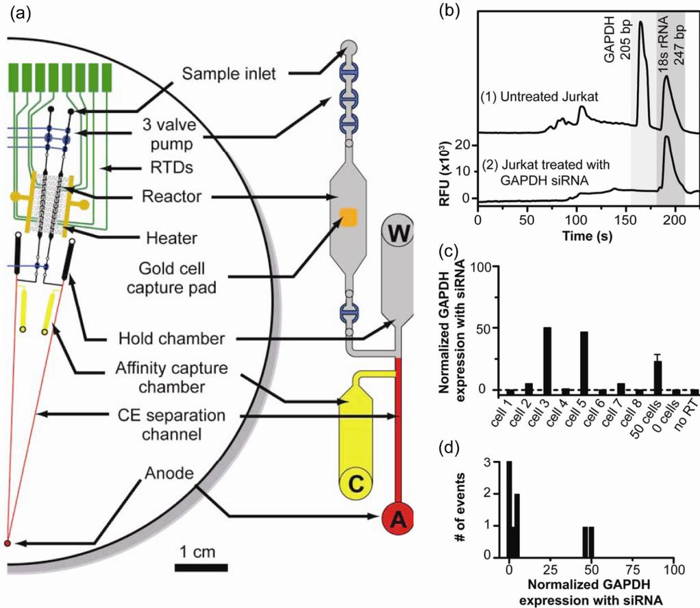
**Figure 2.3.** An integrated microdevice for gene expression analysis of single cells.
