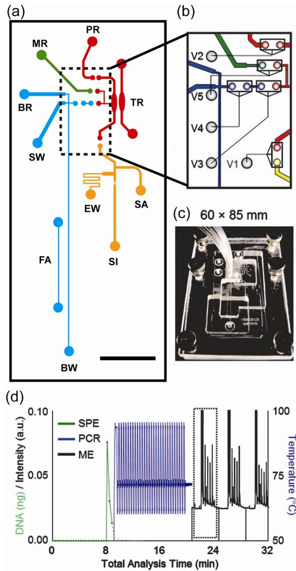
**Figure 2.4.** A fully integrated microfluidic genetic analysis system for pathogen detection.
