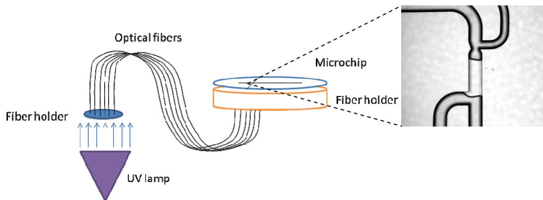
**Figure 6.3.** Schematic of the high-throughput UV exposure system.
