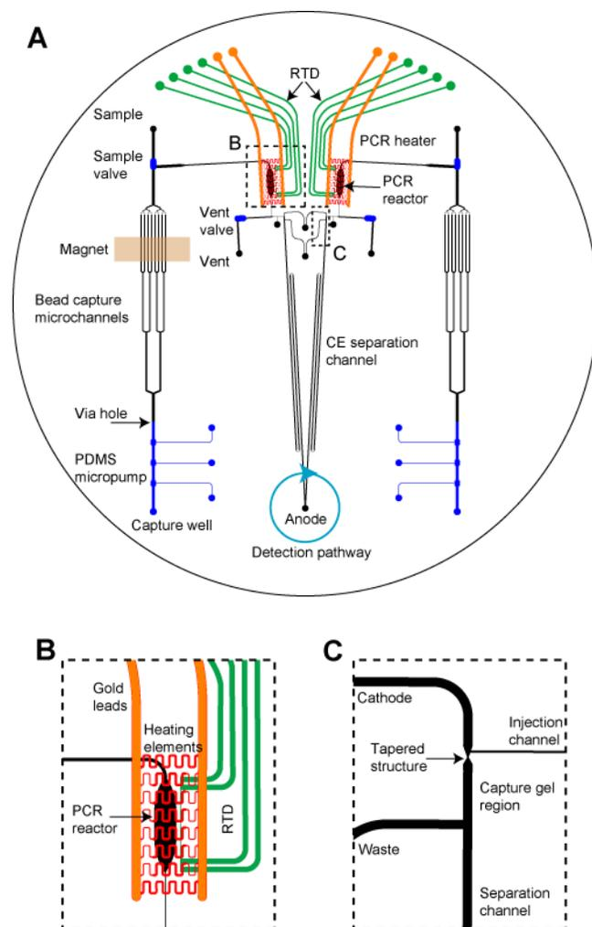
**Figure 5.1.** The design of the fully integrated microdevice for forensic STR analysis.
