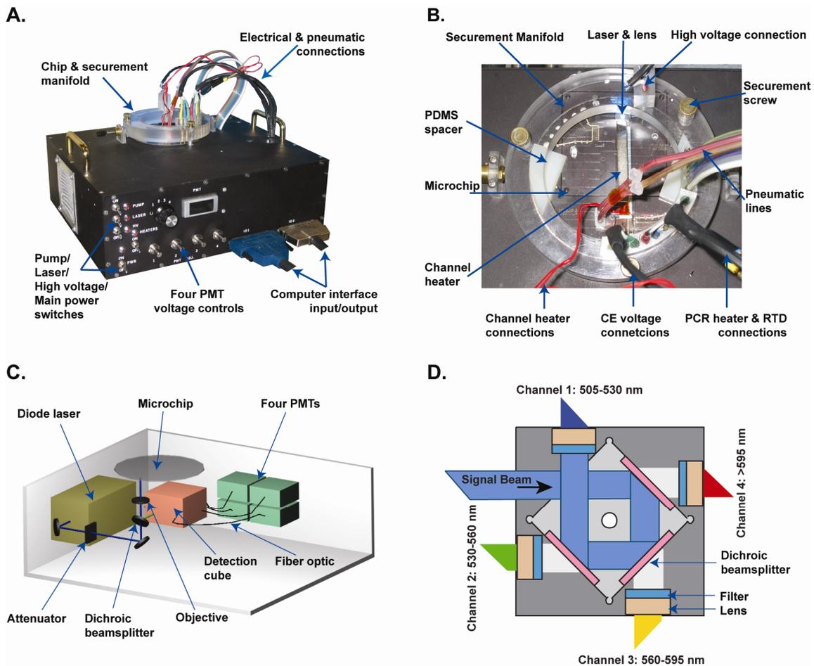
**Figure 3.3.** The structure of the portable instrument.
