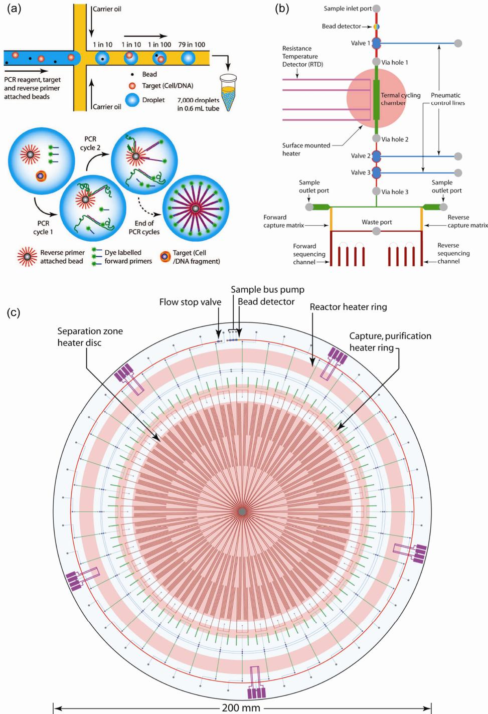
**Figure 2.2.** Integrated high-throughput nanoliter-scale bioprocessor for 100-attomole DNA sequencing generated from single templates in droplets.
