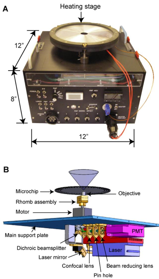
**Figure 5.2.** The structure of the scanner system for chip operation and detection.
