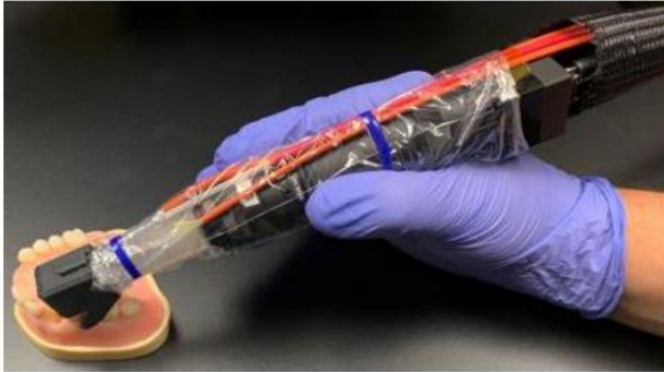
Figure 3. Dual SWIR transillumination/reflectance imaging handpiece.
