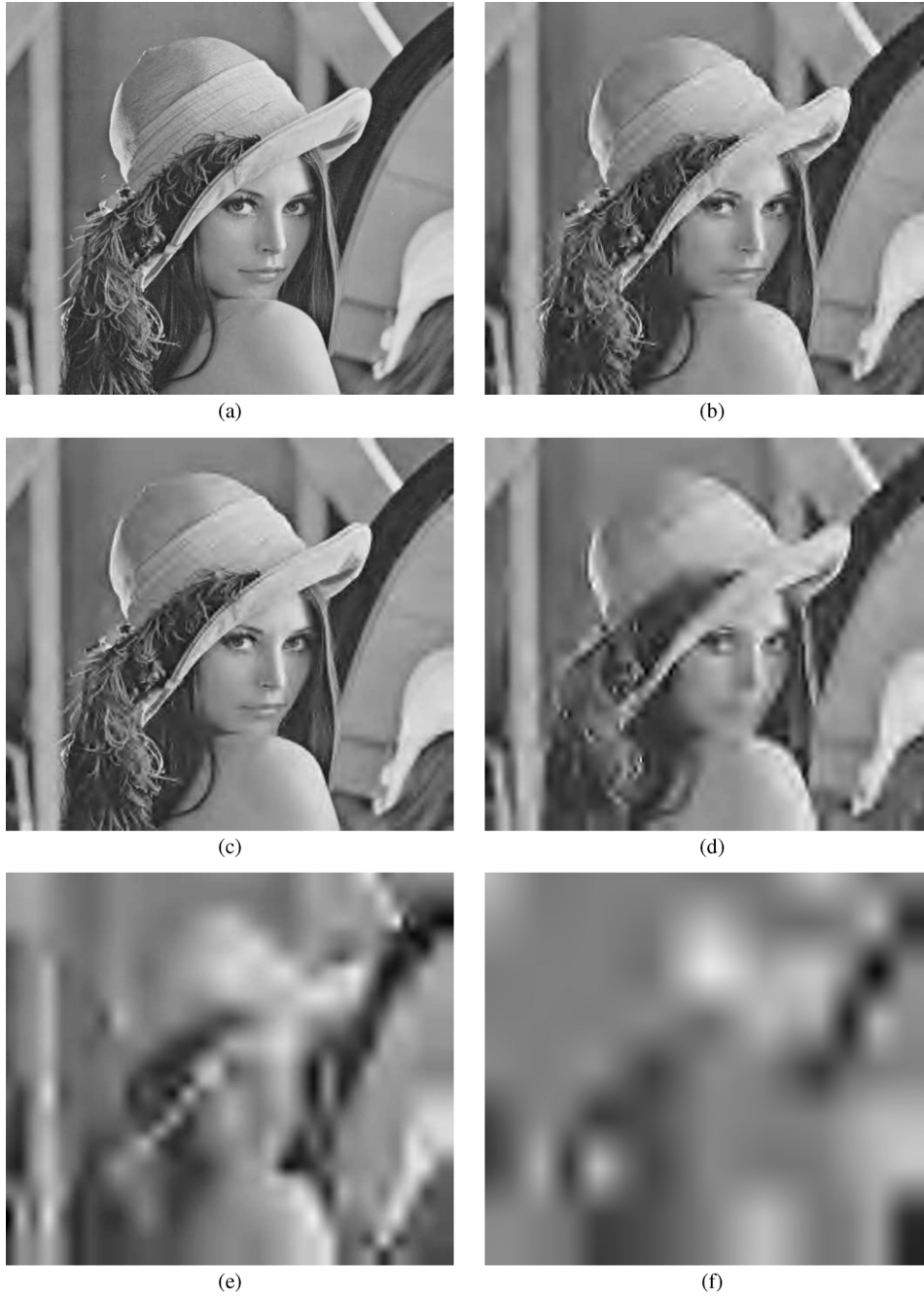
Fig. 12. Image quality for a system with f_{nd} = 10^{-1} , (N, M) = (32, 4) , \text{SNR} = 16 dB, and imperfect CSI. We denote by R_{\text{TX}} the transmitted source rate and by R_{\text{RX}} the received source rate. (a) Original image. (b) Received image. R_{\text{rcpc}} = 0.33 , R_{\text{rs}} = 0.99 , \text{PSNR} = 29.0 dB, R_{\text{TX}} = 0.08 bpp, R_{\text{RX}} = 0.073 bpp. (c) Received image. Optimal Rate. R_{\text{rcpc}} = 0.5 , R_{\text{rs}} = 0.89 , \text{PSNR} = 30.5 dB, R_{\text{TX}} = 0.15 bpp, R_{\text{RX}} = 0.1 bpp. (d) Received image. R_{\text{rcpc}} = 0.66 , R_{\text{rs}} = 0.18 , \text{PSNR} = 25.35 dB, R_{\text{TX}} = 0.03 bpp, R_{\text{RX}} = 0.02 bpp. (e) Received image. R_{\text{rcpc}} = 0.73 , R_{\text{rs}} = 0.03 , \text{PSNR} = 20.5 dB, R_{\text{TX}} = 0.007 bpp, R_{\text{RX}} = 0.004 bpp. (f) Received image. R_{\text{rcpc}} = 1 , R_{\text{rs}} = 0.008 , \text{PSNR} = 14.5 dB, R_{\text{TX}} = 0.001 bpp, R_{\text{RX}} = 10^{-5} bpp.
