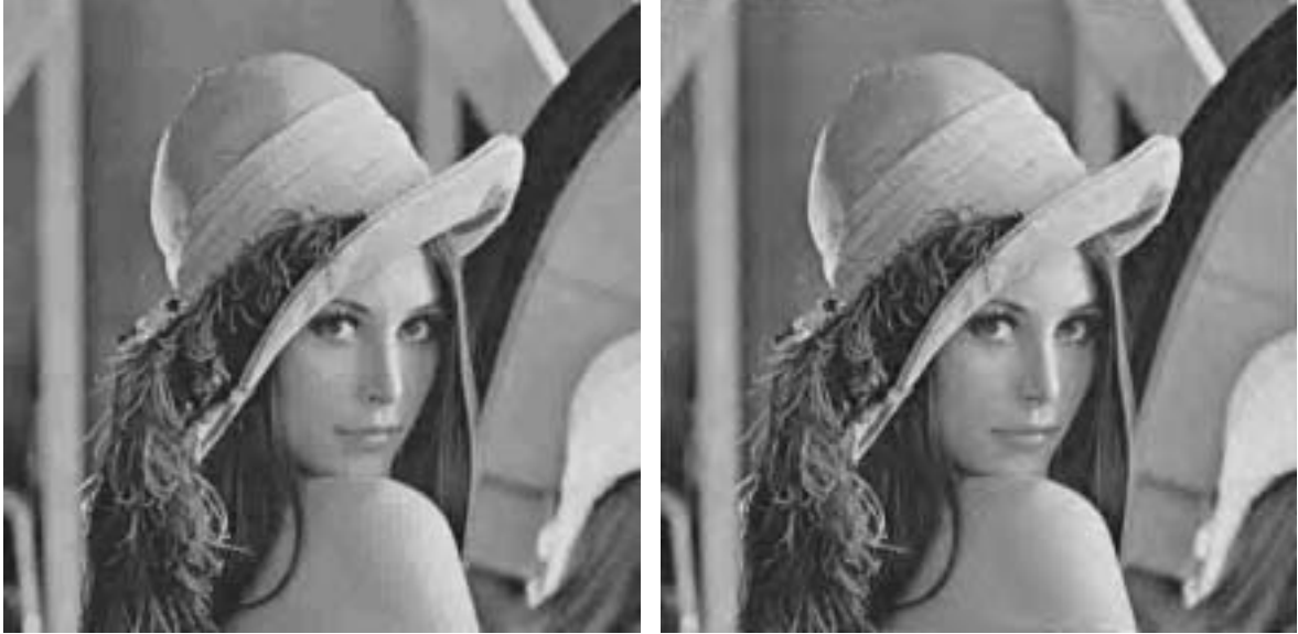
Figure 1: Reconstructed images: (a)left: 0.244bpp by JPEG baseline DCT; (b)right: 0.2bpp by subband or wavelet coder.
