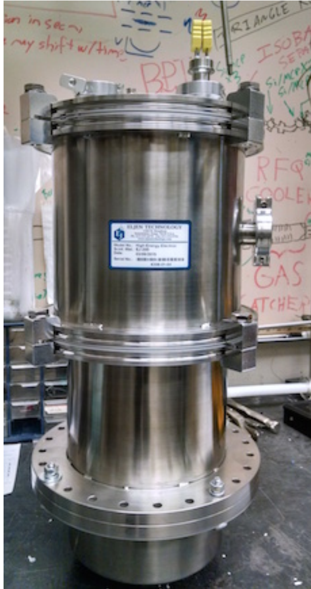
Figure 2.8: An unmounted EJ-200 Plastic Scintillator detector. The scintillating material is located near the bottom of the stainless steel enclosure “can” and the PMT is located near the middle.
