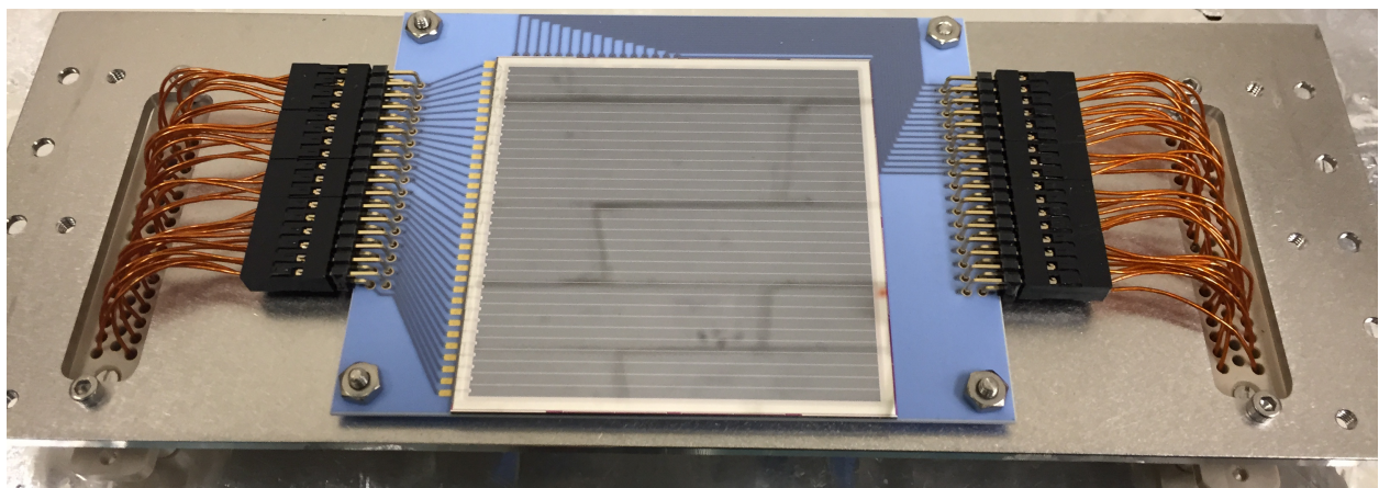
Figure 4.3: A DSSD. The white lines are the insulating edges separating the strips.
