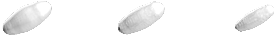
Figure 3.6. Optimization of a distribution analogous to the diagonal points force distribution in 2 dimensions. An isosurface is shown at 50, 100, and 500 iterations (from left to right).
