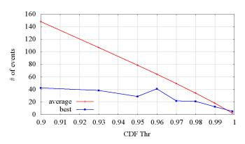
month period from 2007 to 2012. Changing the CDF threshold to 0.9 does not significantly change the number of events either; the average number of events is about 40 with a good set of control parameters for VPIN (blue line) and about 140 with a random set of control parameters (red line).
