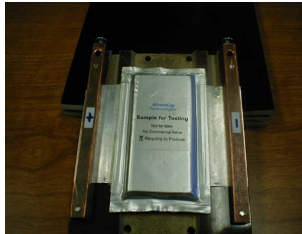
Figure 1: The ApowerCap 450F carbon/carbon device
