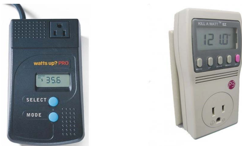
Figure 31. Examples of “plug-through” power meters
