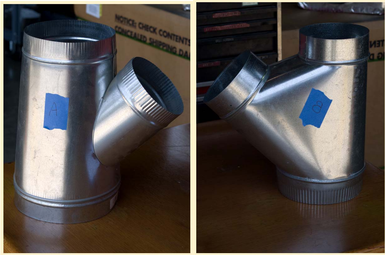
Figure 15. Sheet metal wyes “A” and “B”
