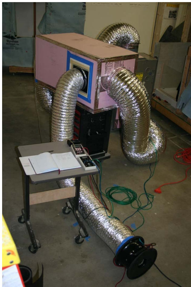
Figure 8. Test chamber connections to furnace and integrated fan/flowmeter
