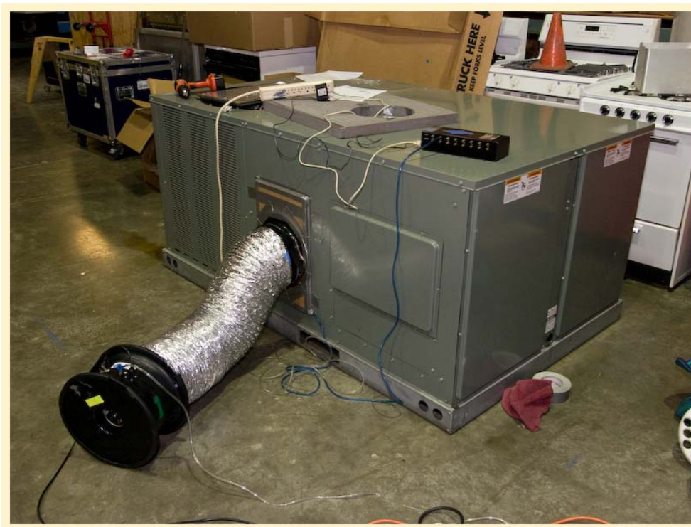
Figure 13. RTU undergoing a pressurization test
