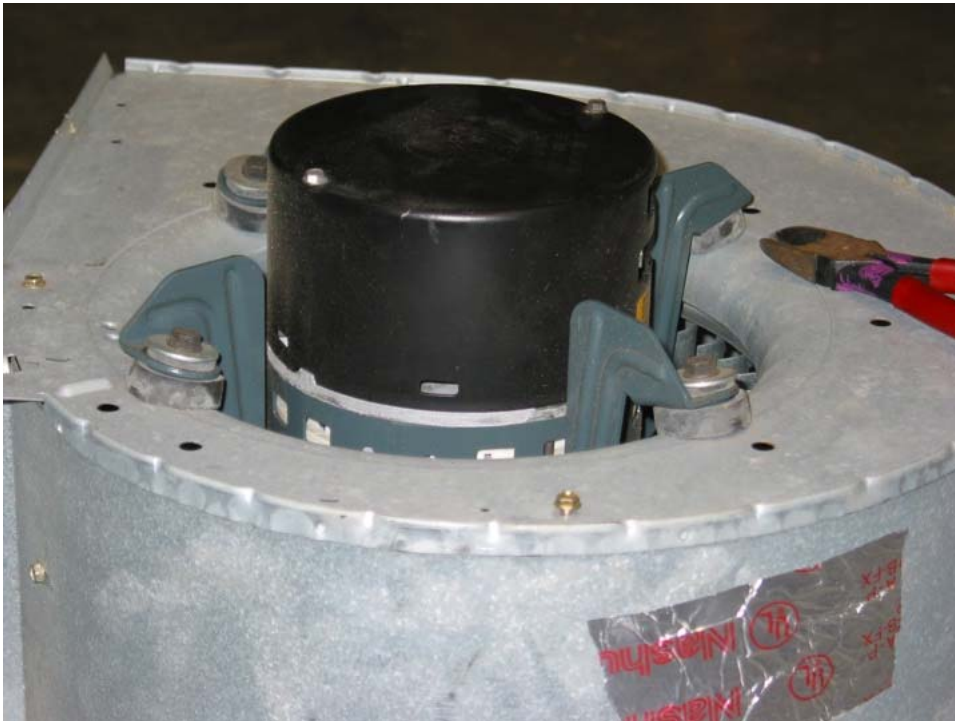
Figure 1. Electric motor protruding from blower inlet that prevents easy air sealing
