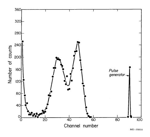
Fig. 3. Spectrum of fragment kinetic energies from spontaneous fission of  ${\rm Cf}^{252}$ . Observed with a solid-state detector reverse-biased by 9 v.
