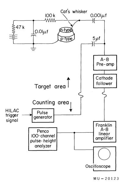
Fig. 2. Electronic system used with the solid-state detectors.
