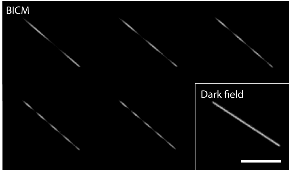
Figure 4.1.5. Typical BICM images of a tethered silicon nanowire. Interpretation of these interference patterns into the inclined angle between the nanowire and a wall and ellipsoidal fitting with the whole nanowire's shape enables tracking of the motion of in 3D. In contrast, such rich information cannot be obtained by dark-field microscopy (right bottom) (scale bar = 10 \mu\text{m} ).
