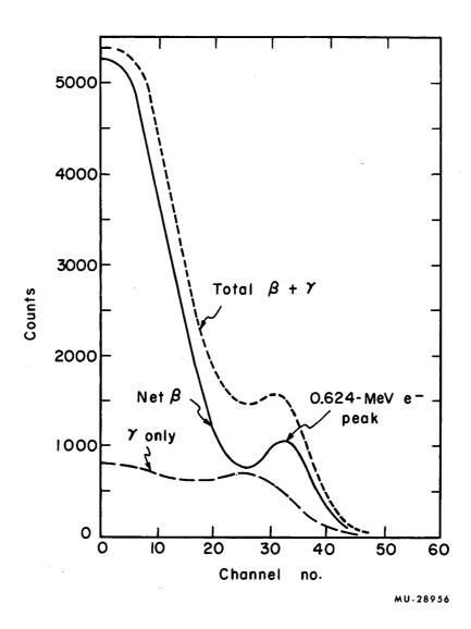
Fig. 10.Cs  $^{137}$  spectra in plastic scintillator ( $2\pi$  geometry). Dotted curve is total counts, dashed curve is background due to the 0.662-MeV  $\gamma$  ray, solid curve is net  $\beta$  spectrum showing the 0.624-MeV conversion peak.
