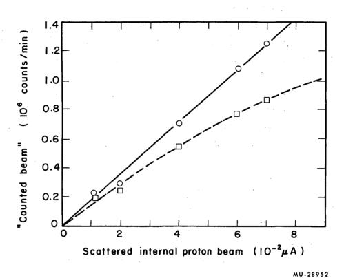
Fig. 6. "Counted beam" versus internal beam. Dashed curve is the uncorrected total counts in telescope. Solid curve is the sum of uncorrected total counts and "accidentals" as defined in the text.
