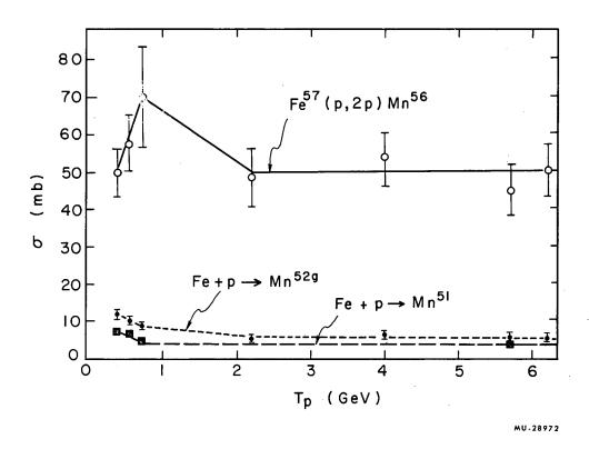
Fig. 30. Excitation functions for production of Mn isotopes from bombardment of natural Fe with protons.
