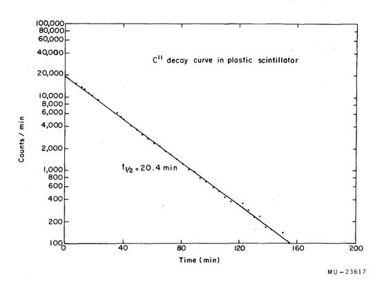
Fig. 13. C<sup>ll</sup> decay curve in plastic scintillator.
