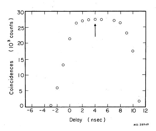
Fig. 3. Delay curve for beam-monitor system. (The arrow represents the optimum operating point.)
