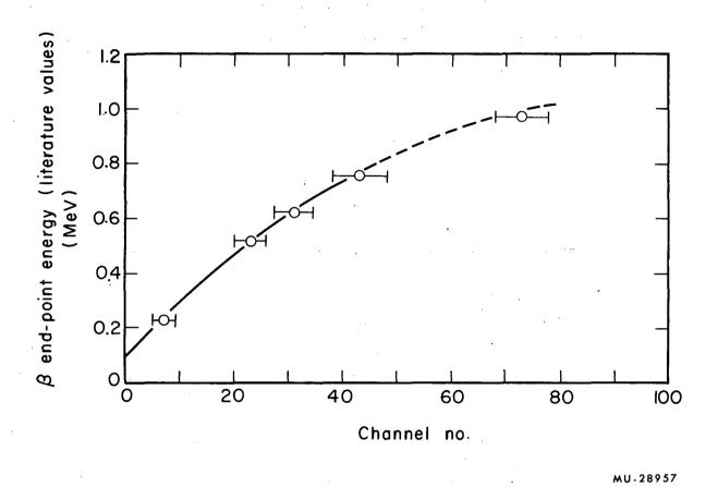
Fig. 12. Calibration curve for  $\boldsymbol{\beta}$  spectra in plastic scintillator.
