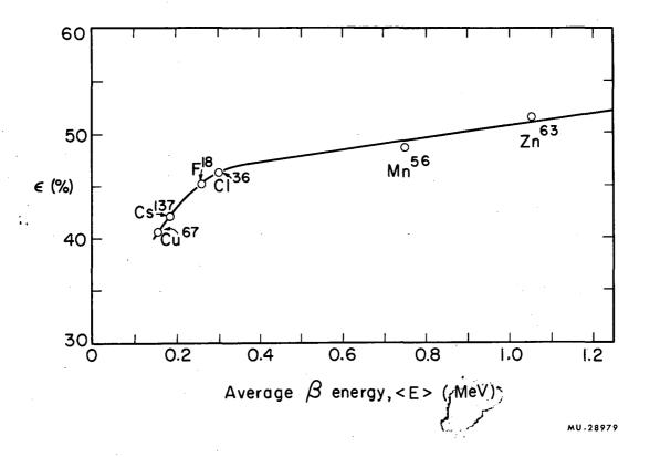
Fig. D-1. Beta-counting efficiency vs average  $\beta$  energy for shelf 1 of end-window proportional counters.  $P^{18}$  point determined by Mahony.  $9^8$  Zn $^63$  point determined by Smith.  $9^8$  Other data are from this work. All efficiencies were determined with weightless sources.
