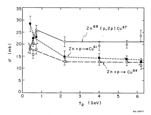
Fig. 29. Excitation functions for production of Cu isotopes from bombardment of Zn with protons.
