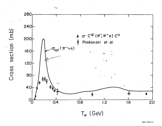
Fig. 17. Cross section for  $C^{12}(\pi^-,\pi^-n)C^{11}$  reaction plotted vs incident pion energy. The smooth curve is the total cross section for  $\pi^-n$  free-particle scattering, which is equal to the total cross section for  $\pi^+p$  scattering by charge symmetry.
