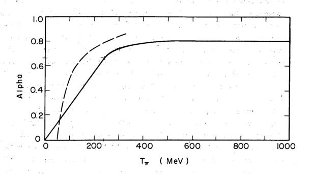
Fig. 25.  $\alpha$  (defined in text) plotted vs incident pion energy. Solid curve is used to calculate pion mean free path. Dashed curve is hypothetical  $\alpha$  if pion-nucleon scattering were isotropic and nonrelativistic.
