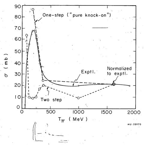
Fig. 28. Comparison of experimental and calculated  $C^{12}(\pi^-,\pi^-n)C^{11}$  excitation functions. Solid curve is experimental. Dashed curve connects the cross sections calculated on the one-step model. The dotted curve connects the points calculated on the two-step model. Both calculated curves have been normalized to the experimental curve at 1610 MeV.
