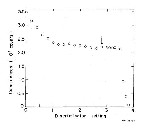
Fig. 5. Discriminator curve. A and B coincidence counts plotted vs discriminator height (arbitrary units).
