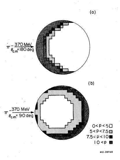
Fig. 26. Location of  $(\pi^-,\pi^-n)$  events from one-step model. This picture of the  $C^{12}$  nucleus represents a plane parallel to the beam path and through the center of the nucleus. p is the relative probability of  $(\pi^-,\pi^-n)$  event calculated from  $p_{ij} = (P_i P_i P_i)_{ij}$ .
