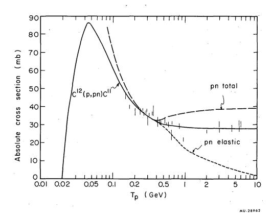
Fig. 19. Solid curve is the C<sup>12</sup>(p,pn)C<sup>11</sup> excitation function plotted from data of references 34,35,36,93,94, and 95. The vertical lines represent the experimental cross sections measured in the high-energy region. Dashed curve is the pn total cross section. Dotted curve is the pn elastic cross section.
