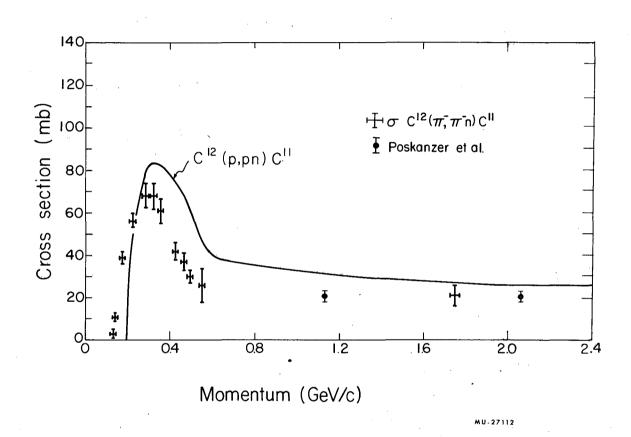
Fig. 20. Cross section for  $c^{12}(\pi^-,\pi^-n)c^{11}$  reaction plotted vs the momentum of the incident pion. The smooth curve is the cross section for  $c^{12}(p,pn)c^{11}$  reaction plotted vs incident proton momentum. Data are taken from references 34,35,36,93,94, and 95.
