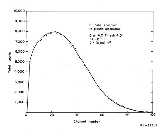
Fig. 11.  $C^{11}$   $\beta$  spectrum in plastic scintillator. The arrow refers to the discriminator cutoff for the scaler.
