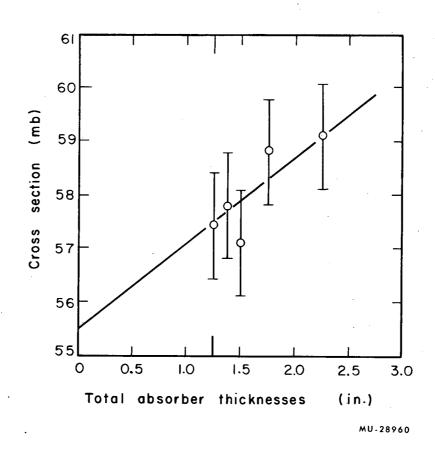
Fig. 15. Correction for finite target thickness.  $C^{12}(\pi^-,\pi^-n)C^{11}$  cross section is plotted vs the sum of the scintillator target, counter B, and lucite thicknesses.
