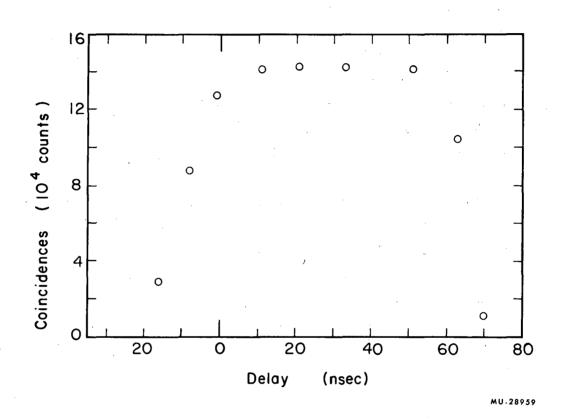
Fig. 15. Delay curve for fast coincidence circuit in  $\beta\gamma$  coincidence experiment.
