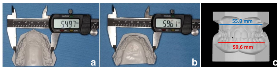
Fig. 1 Measurement of maxillary (a) and mandibular width (b) with a digital caliper on the stone models. The frontal view of maxillary (blue line) and mandibular width (red line) is shown in (c). In this patient, the maxillary width is 55.0 mm, the mandibular width is 59.6 mm, and the maxillary transverse deficiency is 4.6 mm (59.6 – 55.0). The amount of maxillary skeletal expansion required for the patient is equal to the maxillary transverse deficiency (4.6 mm)
