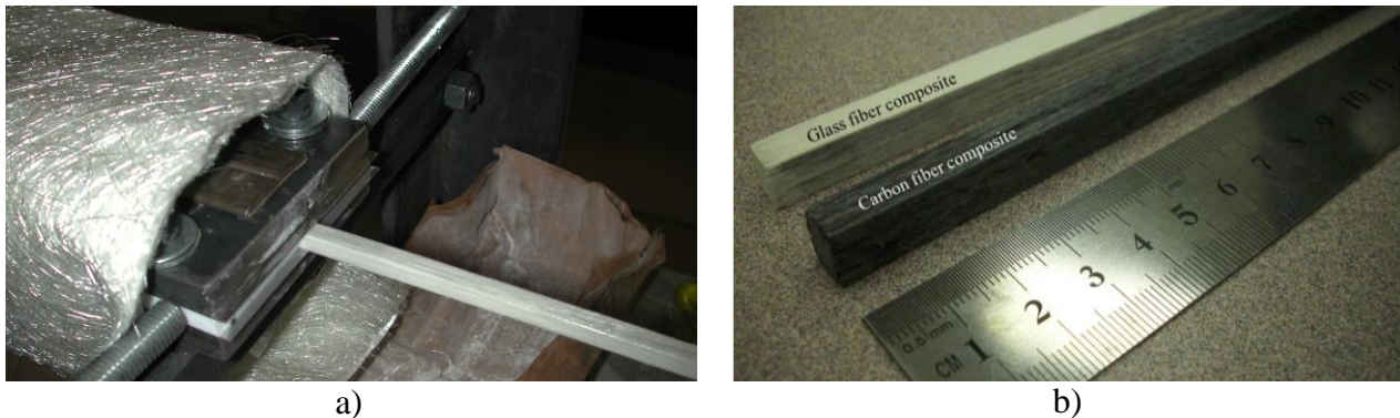
Figure 46 a) pultrusion die during manufacturing of PCs reinforced with unidirectional glass fibers, b) and pultruded bars of PCs reinforced with glass fibers (white) and with carbon fibers (black).
