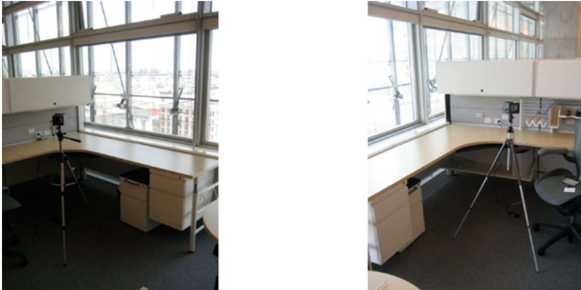
Figure 4.17 Position of HDR camera equipment located in two vacant workstations on the SE facade. East-facing view (left) and south-facing view (right).
