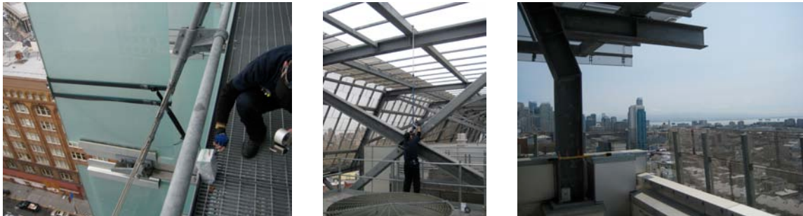
Figure 4.7 Location of exterior solar measures. Vertical illuminance/irradiance on northwest facade (left), rooftop horizontal illuminance/irradiance (center), and vertical illuminance/irradiance on the SE facade (right).
