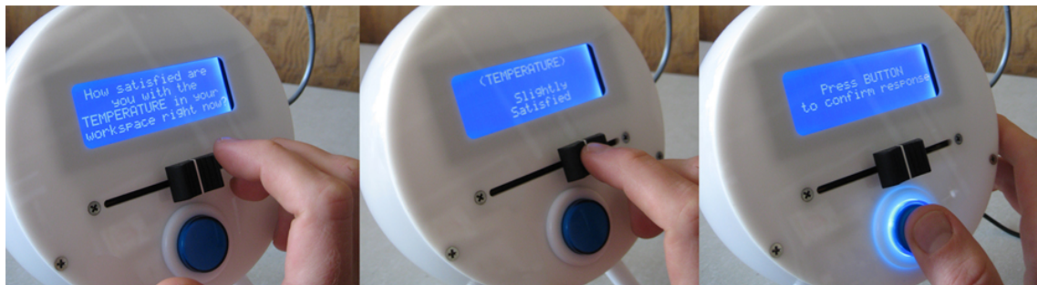
Figure 4.29 Example data entry sequence: (left) IEQ question is displayed to the user on the screen, (center) user selects desired subjective response, (right) after user has selected response arcade button is pressed to record response and advance to next question.
