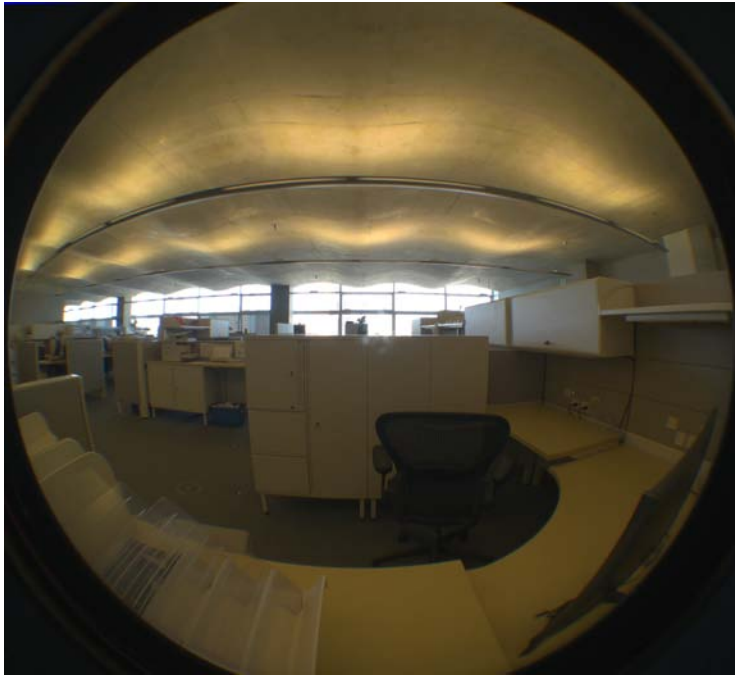
Figure 9.11 View from core workspace to NW facade showing potential loss of view as a result of high contrast between windows and surrounding interior surfaces.
