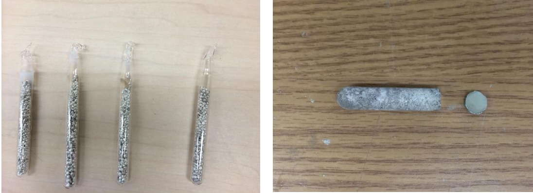
Fig. 2.7 Metal shots before casting (left) and grown ingot (right) after casting.
