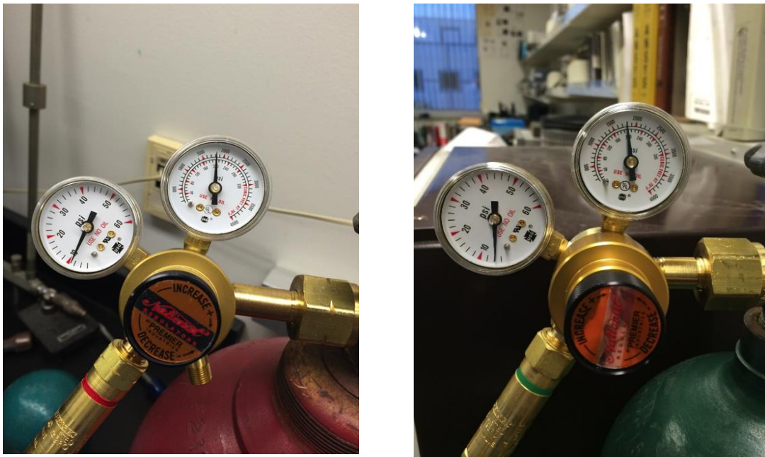
Fig. 2.3 Normal pressures of gauges for hydrogen cylinder (left) and for oxygen cylinder (right) at working status.
