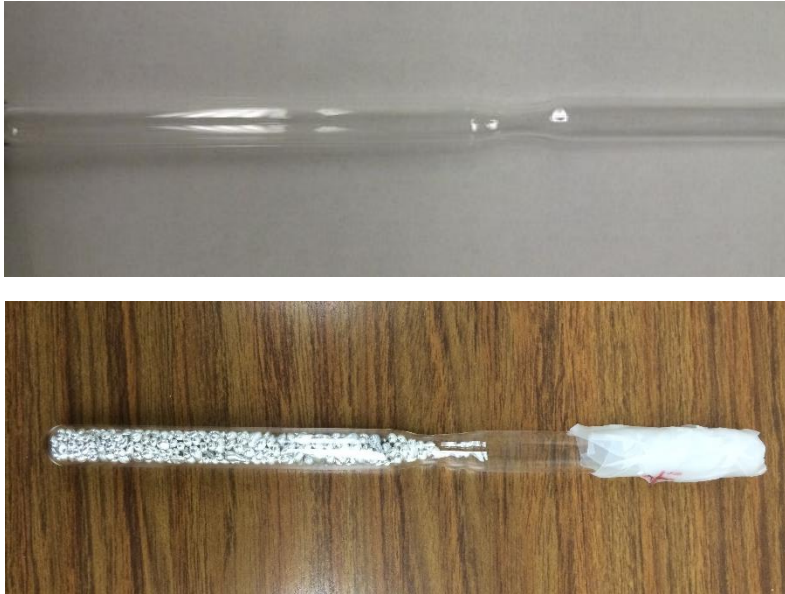
Fig. 2.4 The picture of quartz tube (top) and filled with metallic shots (bottom).
