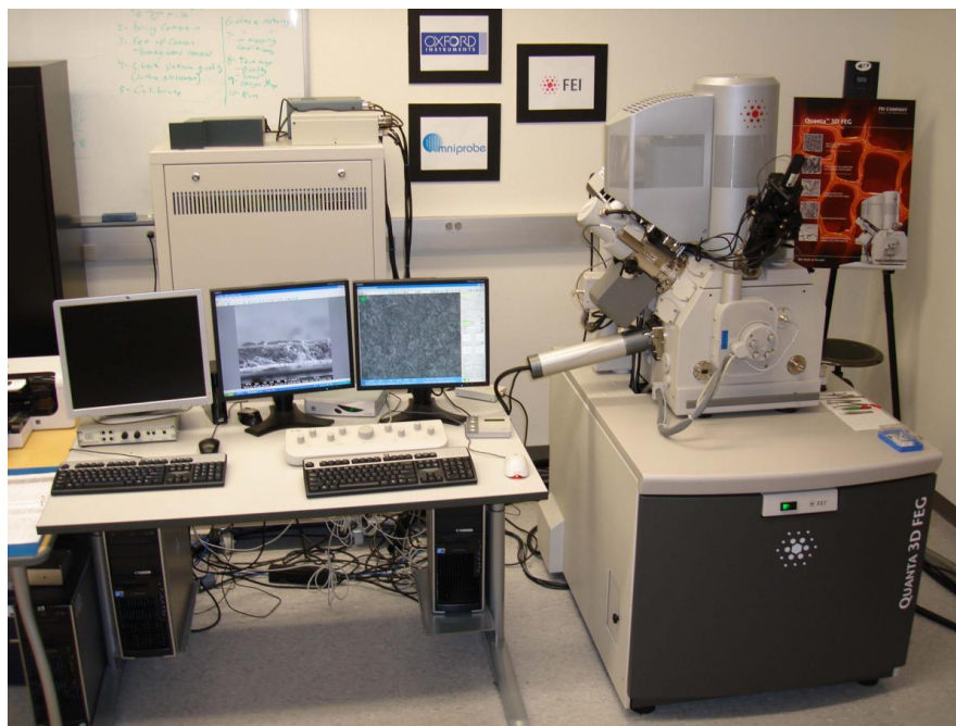
Fig. 2.22 FEI Quanta 3D FEG Dual Beam SEM/FIB Instrument.
