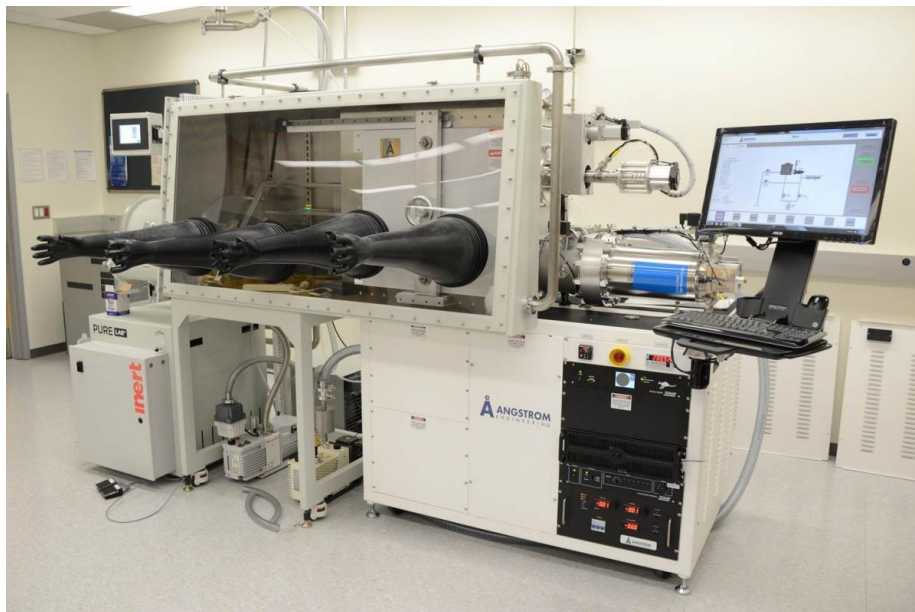
Fig. 2.9 Angstrom Engineering EvoVac Glovebox Evaporator.
