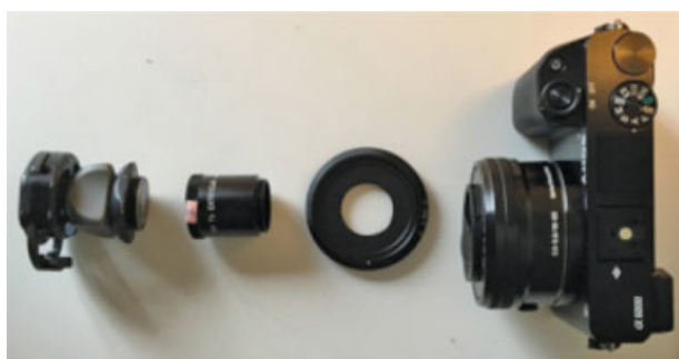
Fig. 1 Digital endoscopic equipment (from right to left): a6000 mirrorless camera (Sony Inc.), C-Nex mount adapter, 5X extender and the coupler (Stryker).
