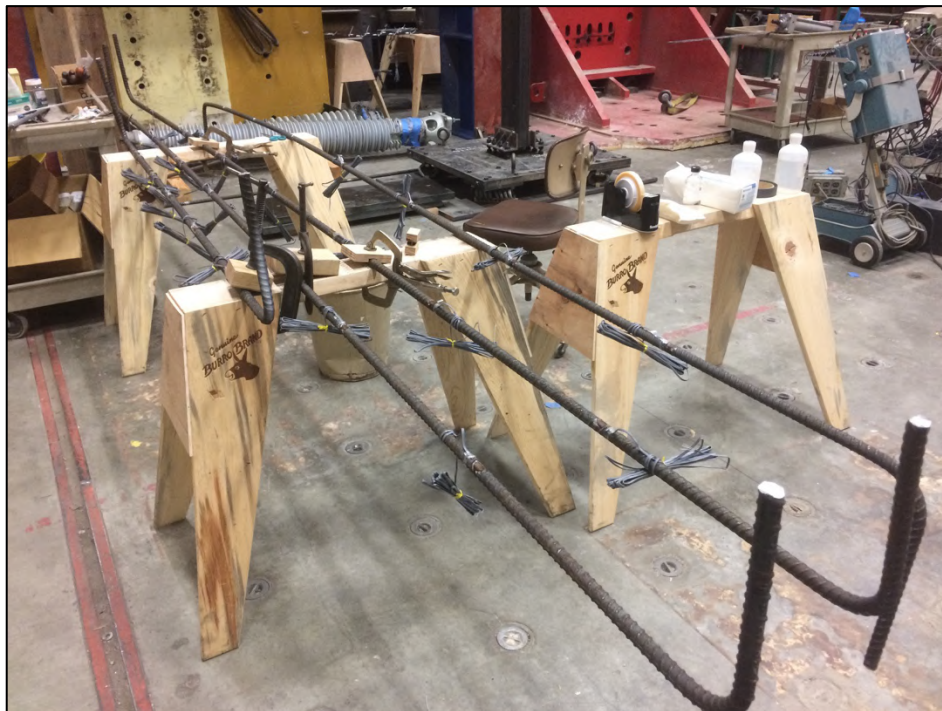
Figure G- 14. Installation of strain gages #2
