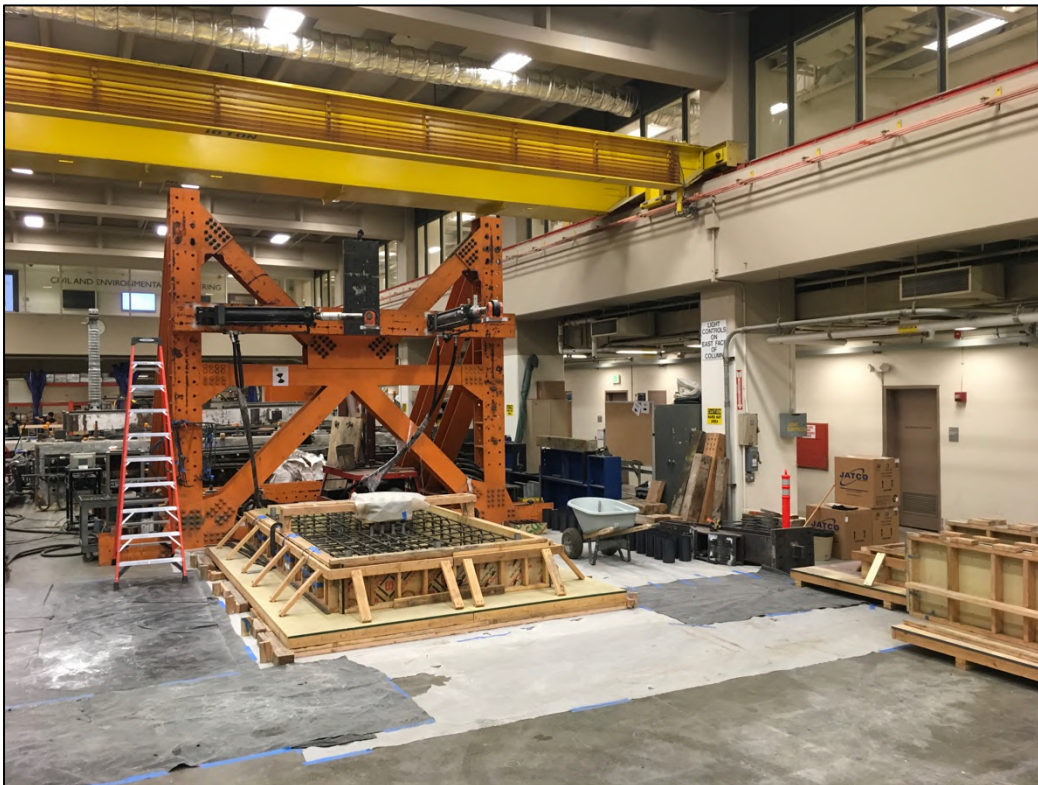
Figure G- 19. Specimen form with reinforcement ready to cast #3
