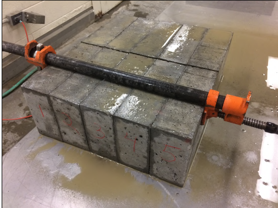
Figure G- 46. Madium fracture energy beams held together and saw cut
