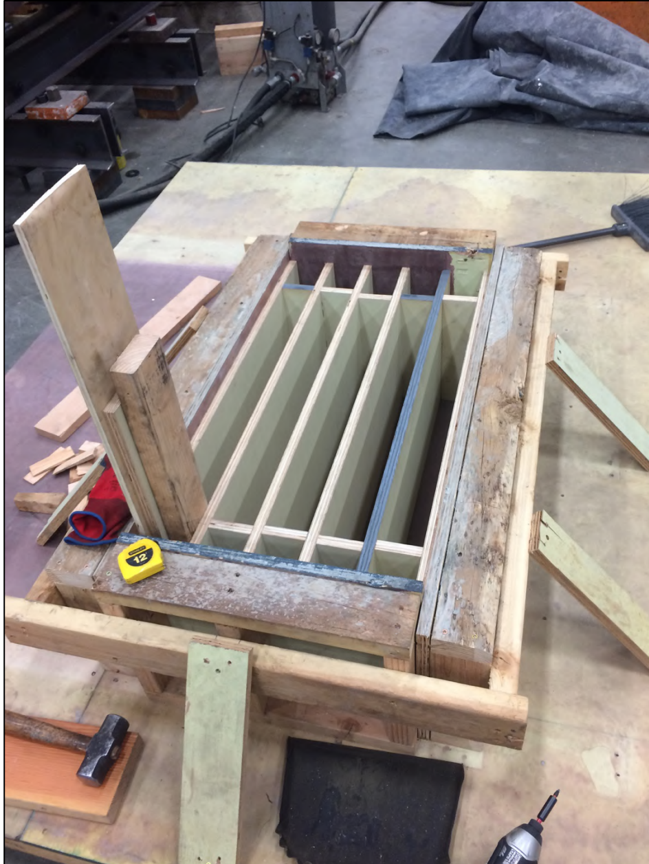
Figure G- 41. Construction of fracture energy molds for large beams
