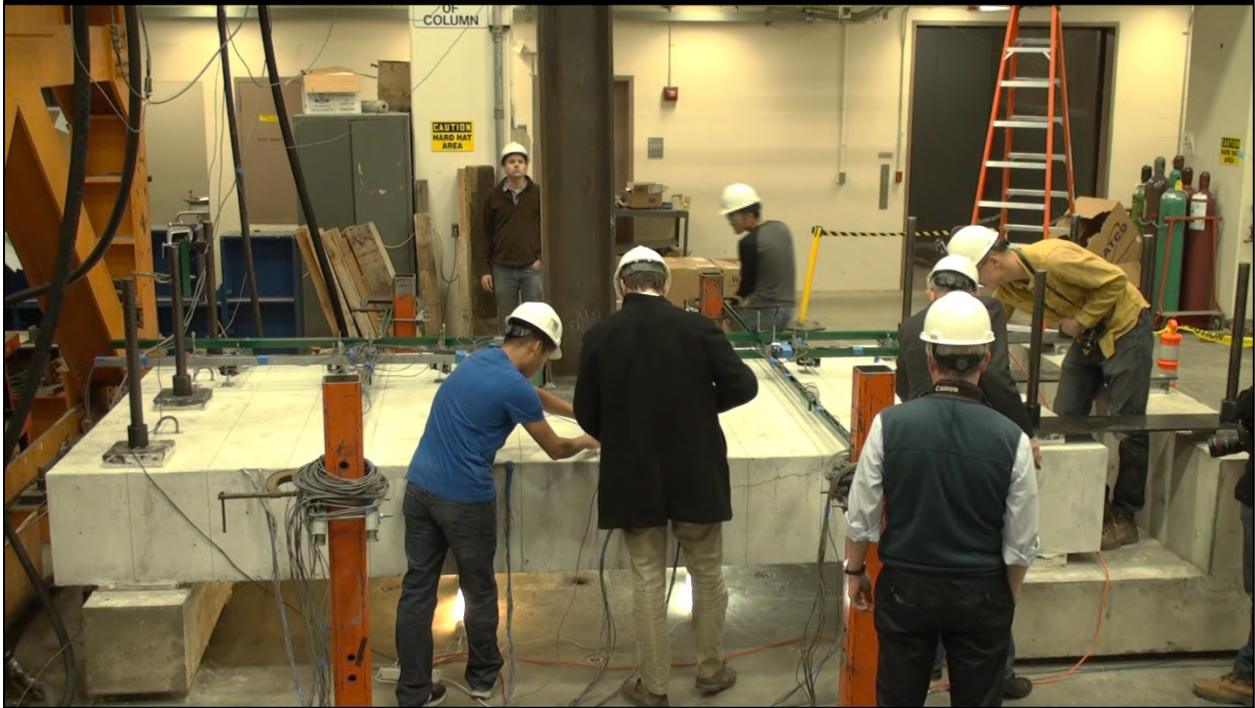
Figure G- 36. Crack marking during a pause while testing December 12, 2017
