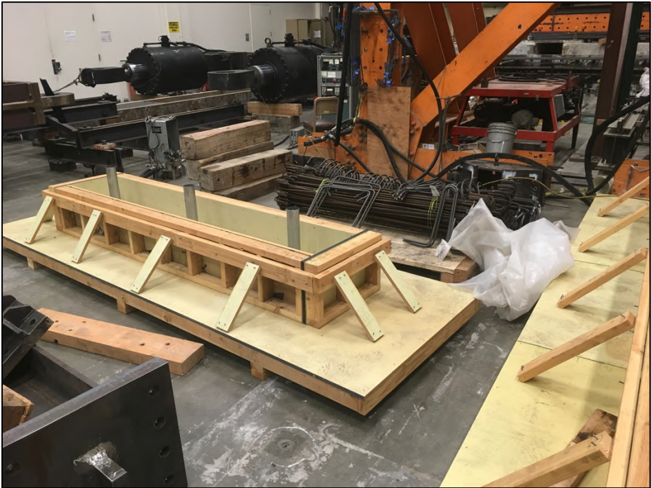
Figure G- 2. Support type 2 form with through holes
