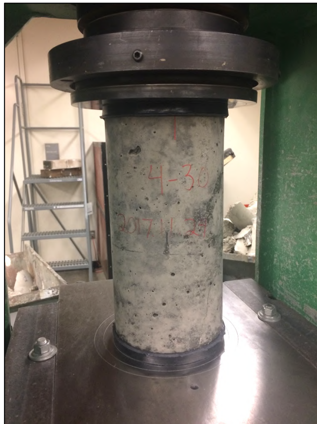
Figure G- 49. Cylinder compression testing
