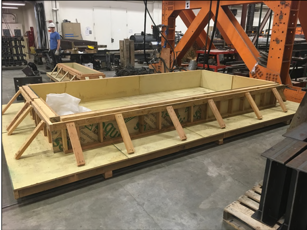
Figure G- 11. Specimen form and support type 2 form in the background
