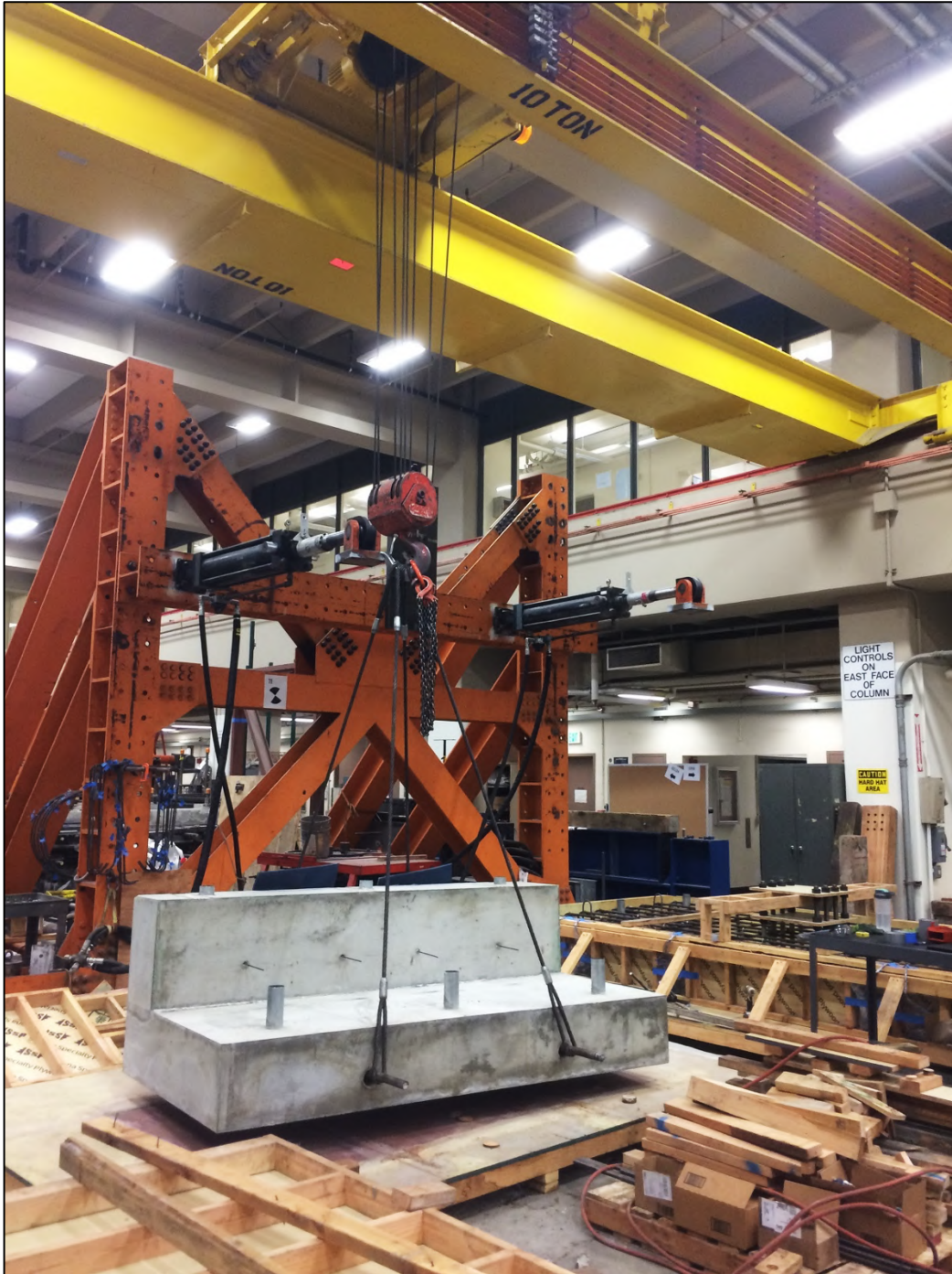
Figure G- 26. Support type 1 demolding
