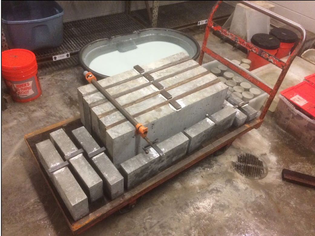
Figure G- 44. Fracture energy beams with top plate attached with hydrostone
