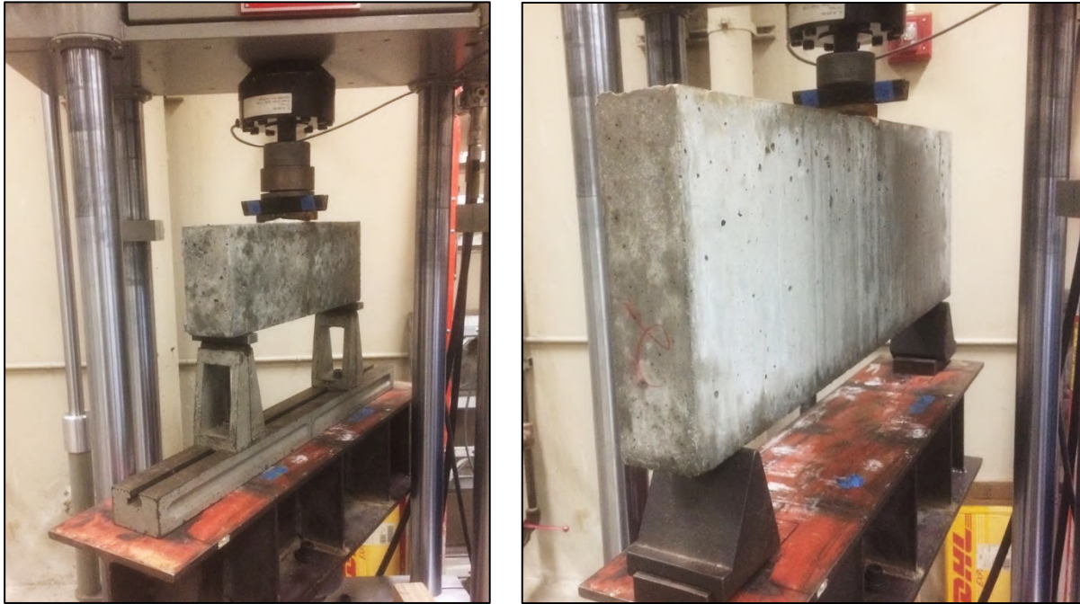
Figure A- 3. Concrete Fracture Energy test set-up
