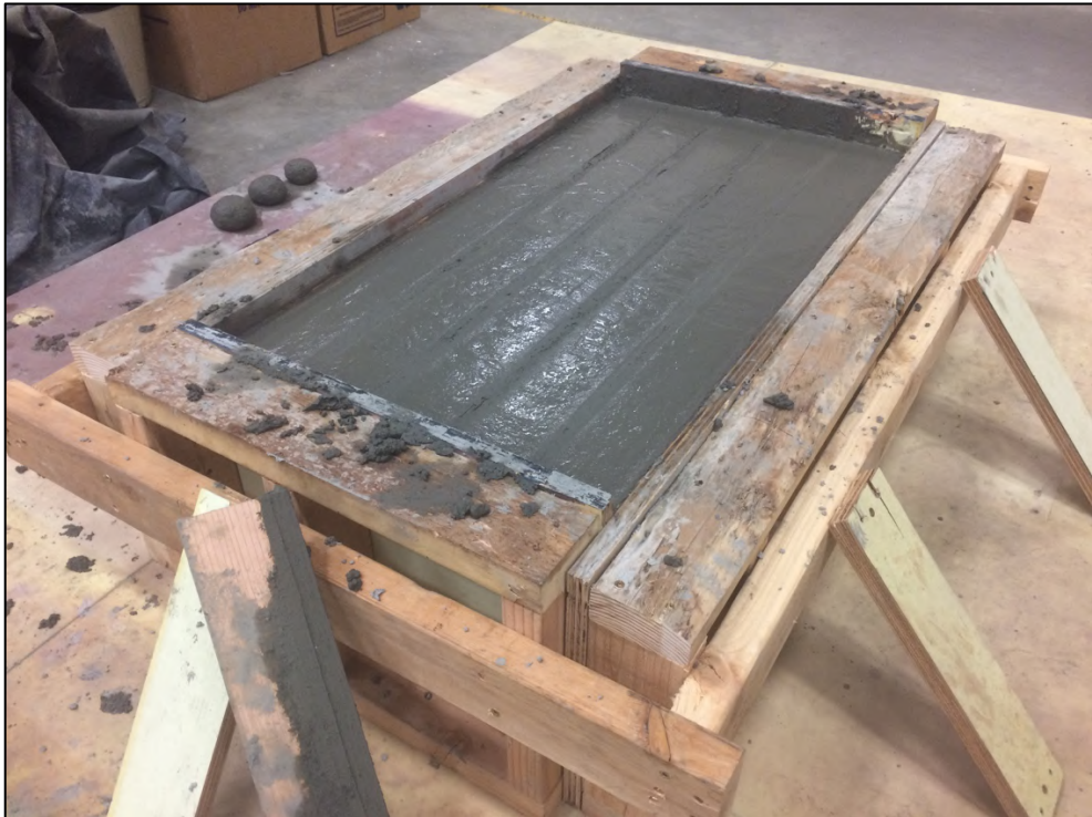
Figure G- 43. Large fracture energy beams hours after casting November 21, 2017
