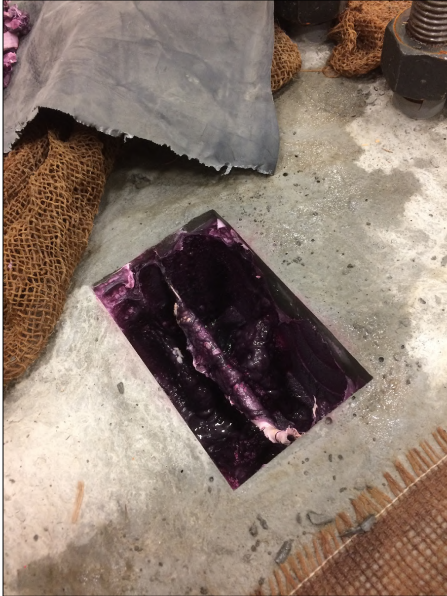
Figure G- 23. Removal of foam from specimen to reveal hole for shear lug #1
