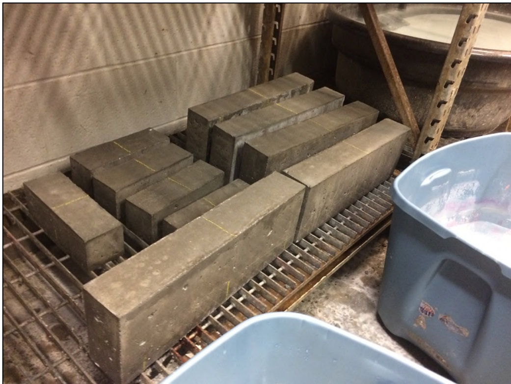
Figure G- 45. Fracture energy beams after removing from lime bath
