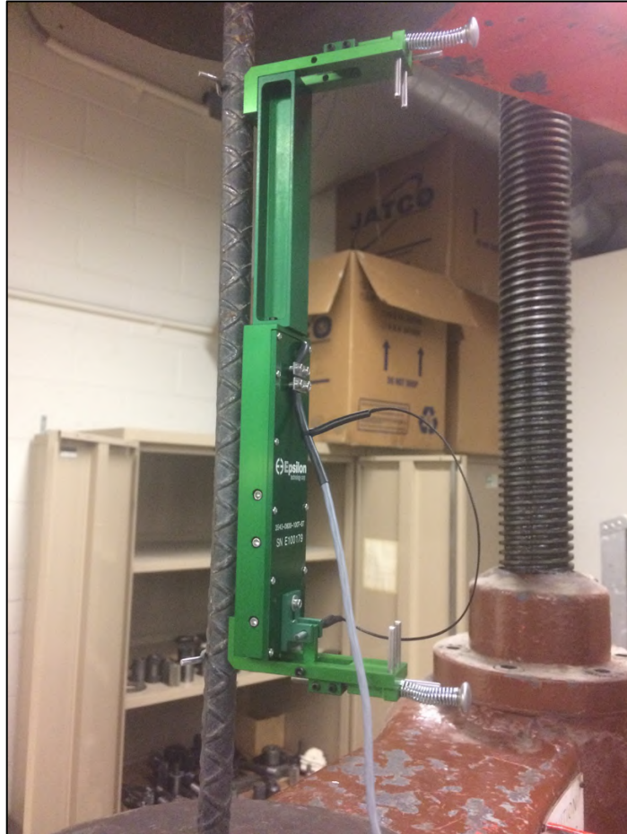
Figure G- 50. Reinforcing bar testing
