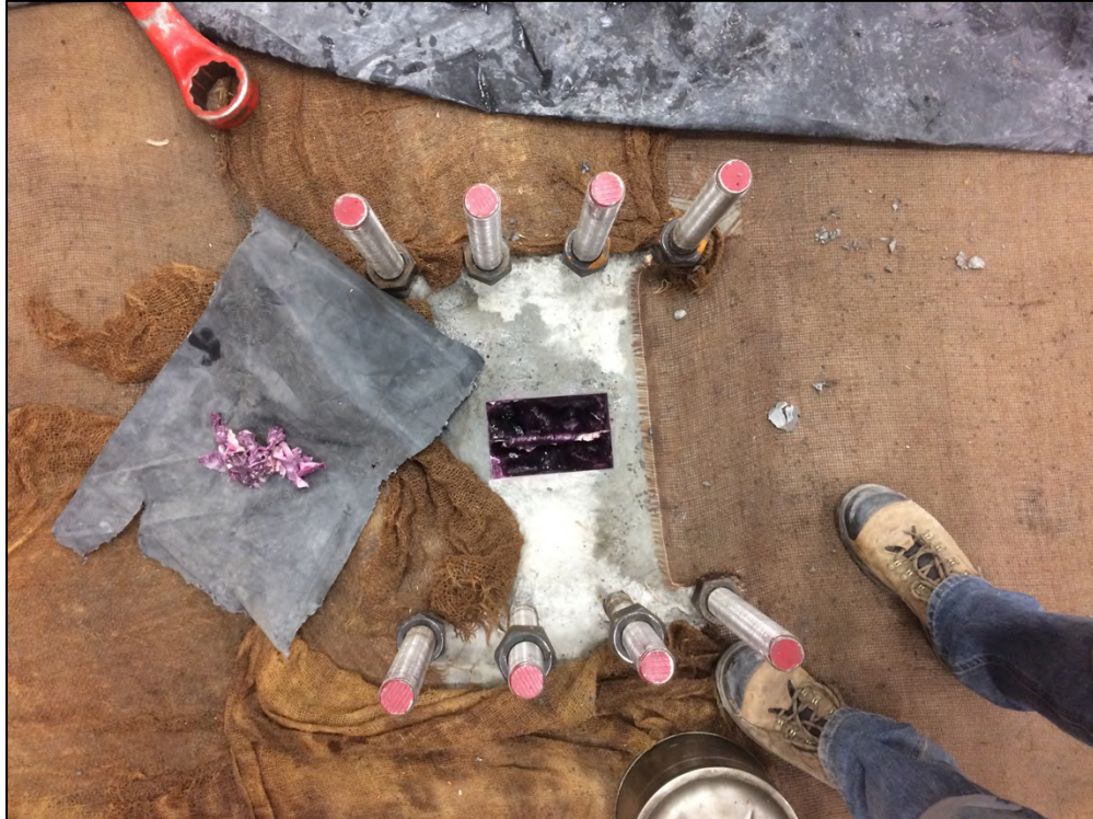
Figure G- 24. Removal of foam from specimen to reveal hole for shear lug #2
