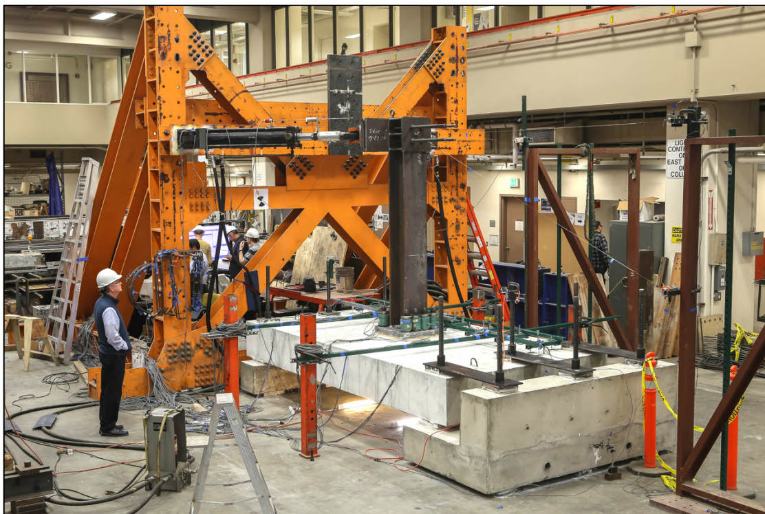
Figure 4-1. Specimen set-up and instrumentation
