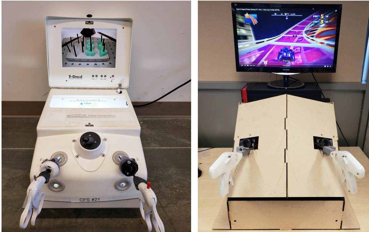
Figure 3.3. Systems used for the study included the 3-Med trainer (left), which was used for training the standard simulator group, as well as for conducting the FLS tests, and the new system proposed here (right) with a non-inverted and an inverted instrument mapping.
