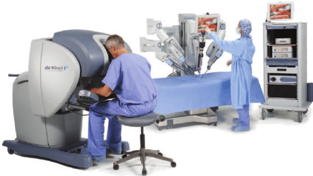
Figure 1.1. This figure, which originally appeared in HWR Schreuder et al. [44], shows the da Vinci S robotic system with a master console and a patient side robot arms(Intuitive Surgical, Inc.)
