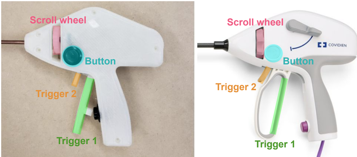
Figure 2.4. Customized instrument for the new system (left) and inputs corresponding to critical inputs on a commercial instrument (right).
