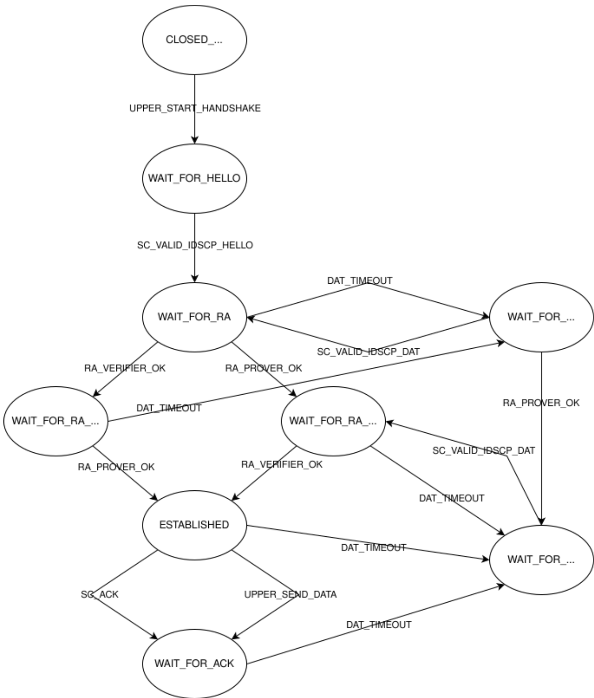
Figure 3.4. Simplified IDSCP2 Finite State Machine [26]
