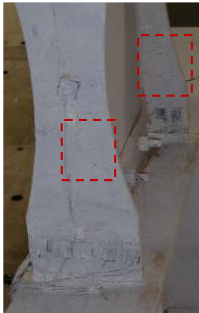
(b) Yielding in Beam Top and Bottom Flanges
