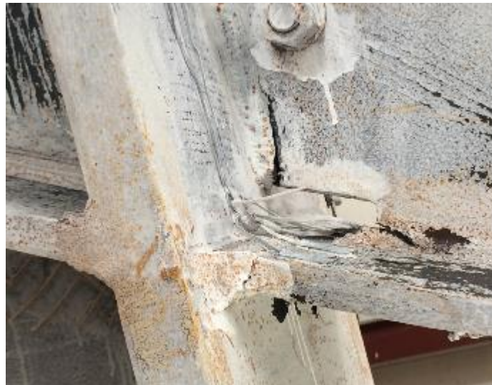
(b) Detail A (Fractures at Beam Web CJP Weld and Weld Access Hole)
