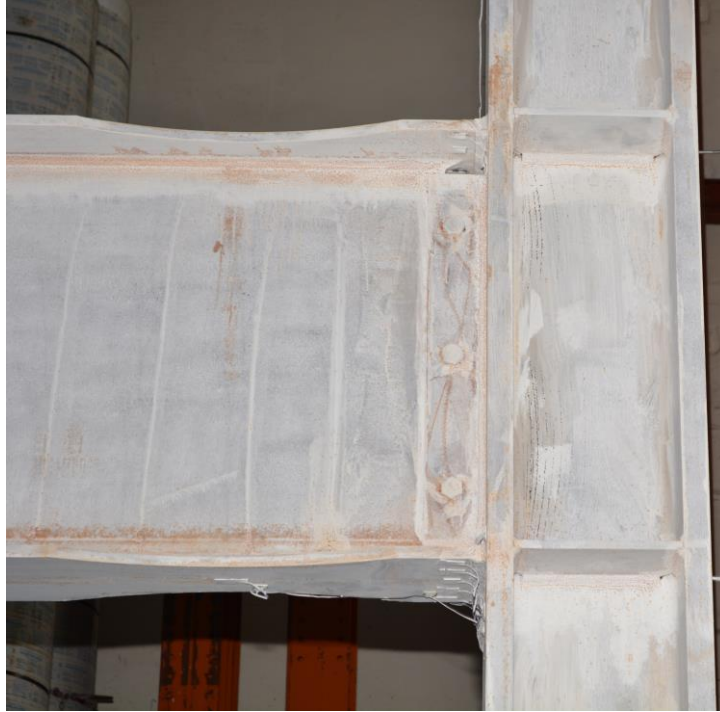
Figure 3.30 Specimen C2 Panel Zone Minor Yielding at Completion of 0.0075 rad Drift Cycles
