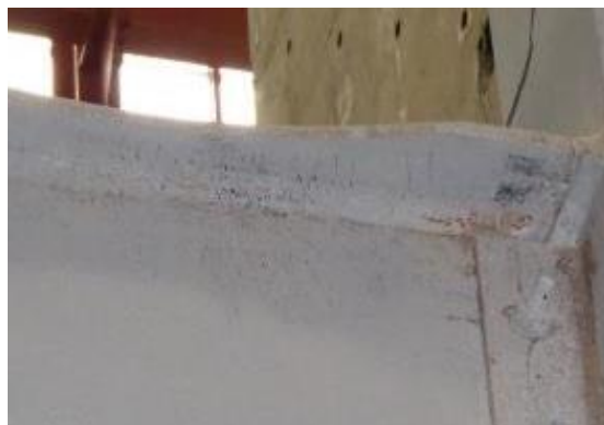
(c) Spread of Yielding to Beam Web
