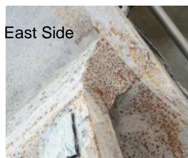
(c) Top Flange CJP Weld (No Fracture)
