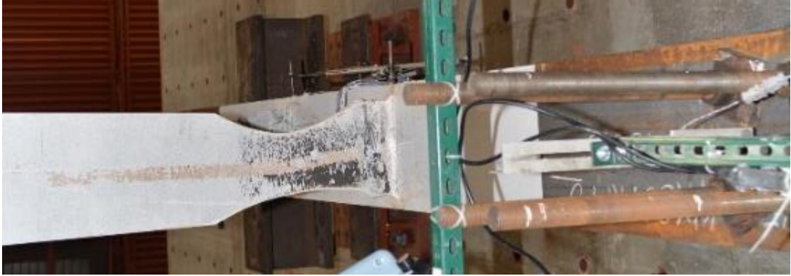
(a) -0.04 rad Drift (1 st Cycle)
