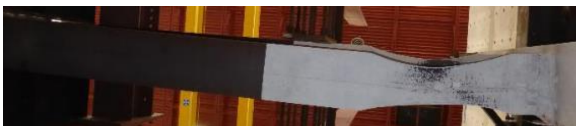
(e) Beam Lateral-Torsional Buckling
