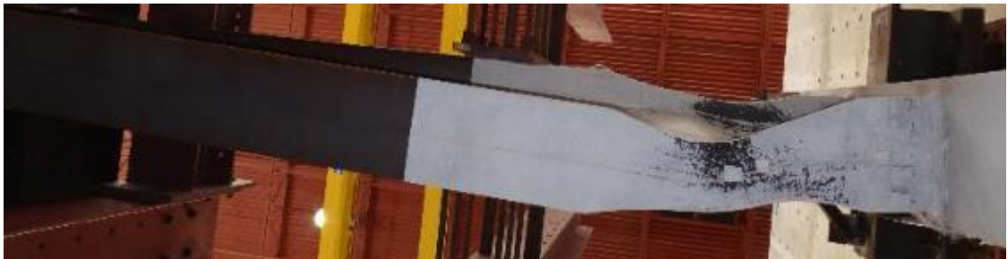
(c) -0.05 rad Drift (1 st Cycle)
