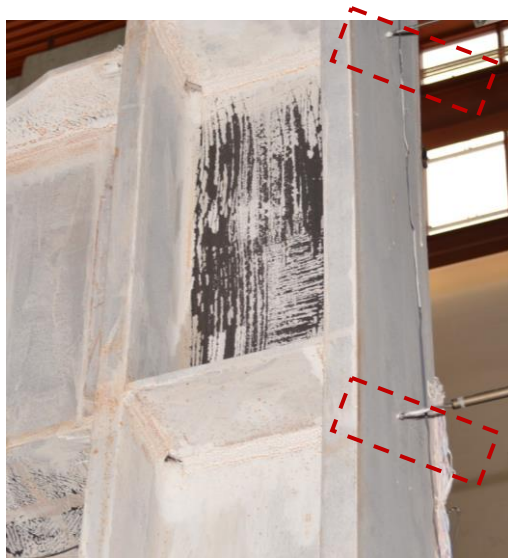
(b) Column Flange Yielding Due to Column Kinking (Back Side)
