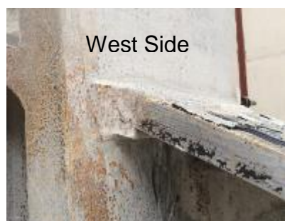
(c) Top Flange CJP Weld (No Fracture)
