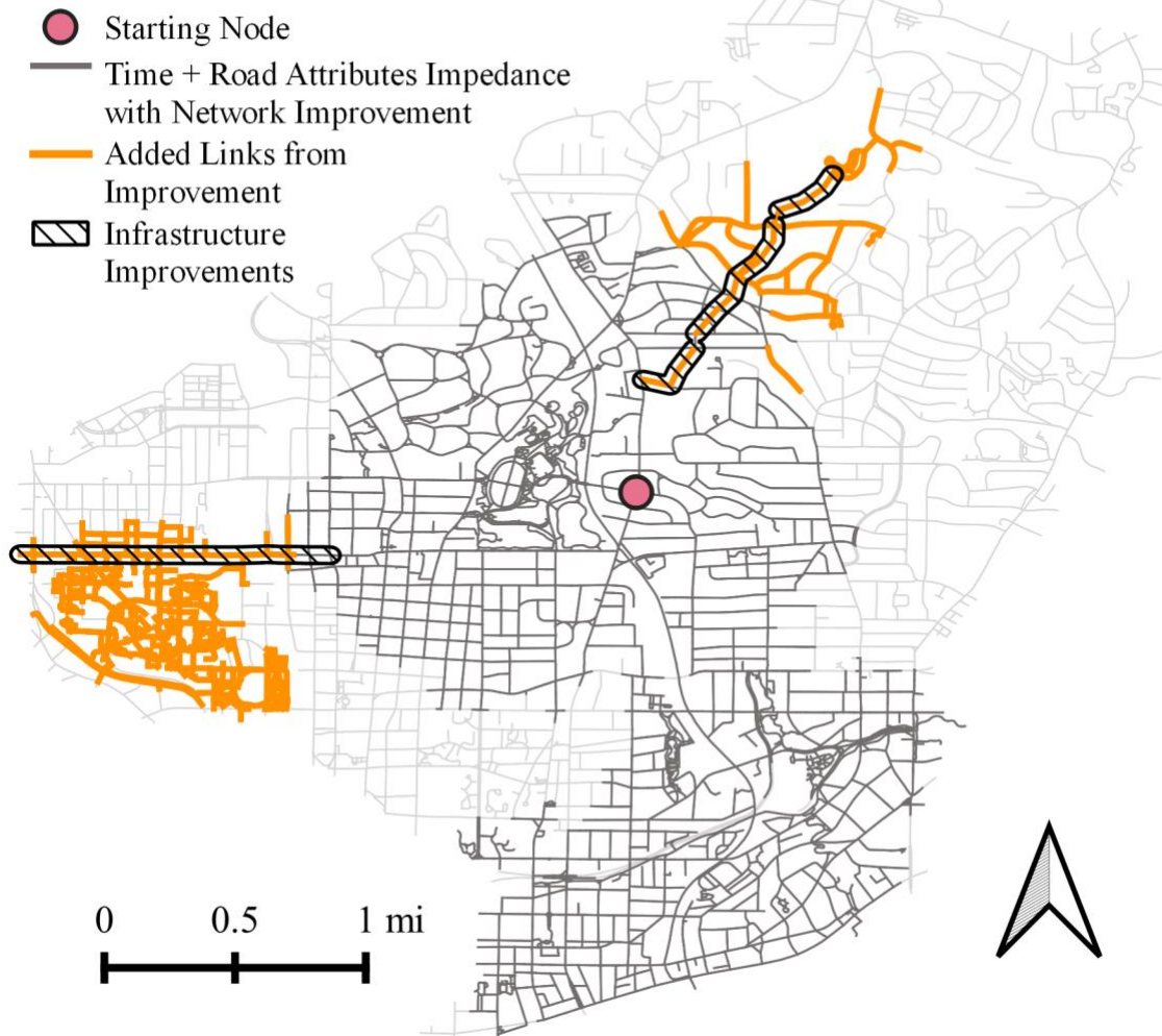
Figure 5. Change in the time + attribute impedance 10-minute bikeshed after two multi-use paths were added to the network
