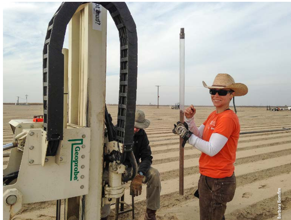
A Geoprobe push-drill system was used to collect soil cores to 30 feet in depth in fields planted in almonds, tomatoes and wine grapes in the Kings groundwater subsbasin.
