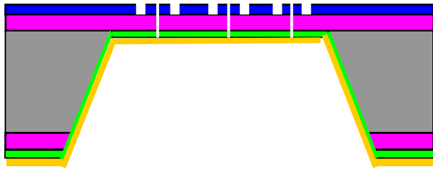
Figure 4.10. Microfabrication process flow for the 2 nd version pattern generator with LSN film
