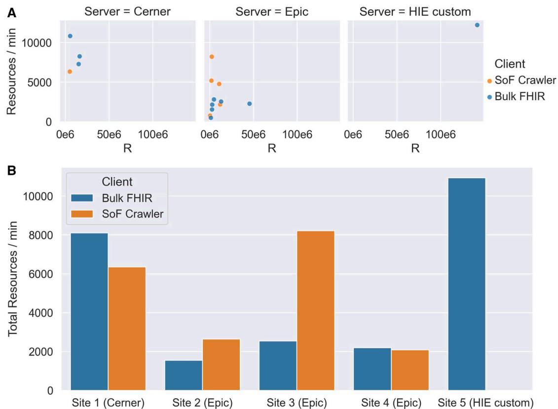
Figure 1. Performance scaling differences between vendors. (A) Measured export speed plotted against total number of resources in each benchmark. (B) Total count of resources exported at each site divided by total export time. Performance is grouped by API service provider. R = total number of resources.
