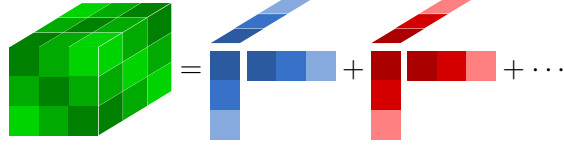
Figure 1.4: CP decomposition of a symmetric 3rd order tensor T = \sum_i a_i \otimes a_i \otimes a_i
