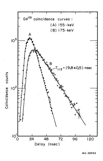
Fig. 2. Gadolinium-151 coincidence curves: (A) 155-21.7 keV "prompt" curve, (B) 175-21.7 keV delay curve. Chances have been subtracted.
