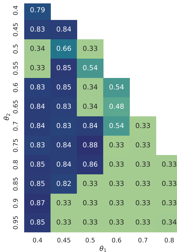
Figure 5: The influence of listener parameters to the accuracy of CG+LI model. Darker indicates better result, and 0.33 is the trivial accuracy since N = 2 in our experiments. Only showing the lower triangle, since \theta_2 \geq \theta_1 in Alg. 1. The best parameters are the triangle region on the center left, and parameters outside it easily lead to failure.
