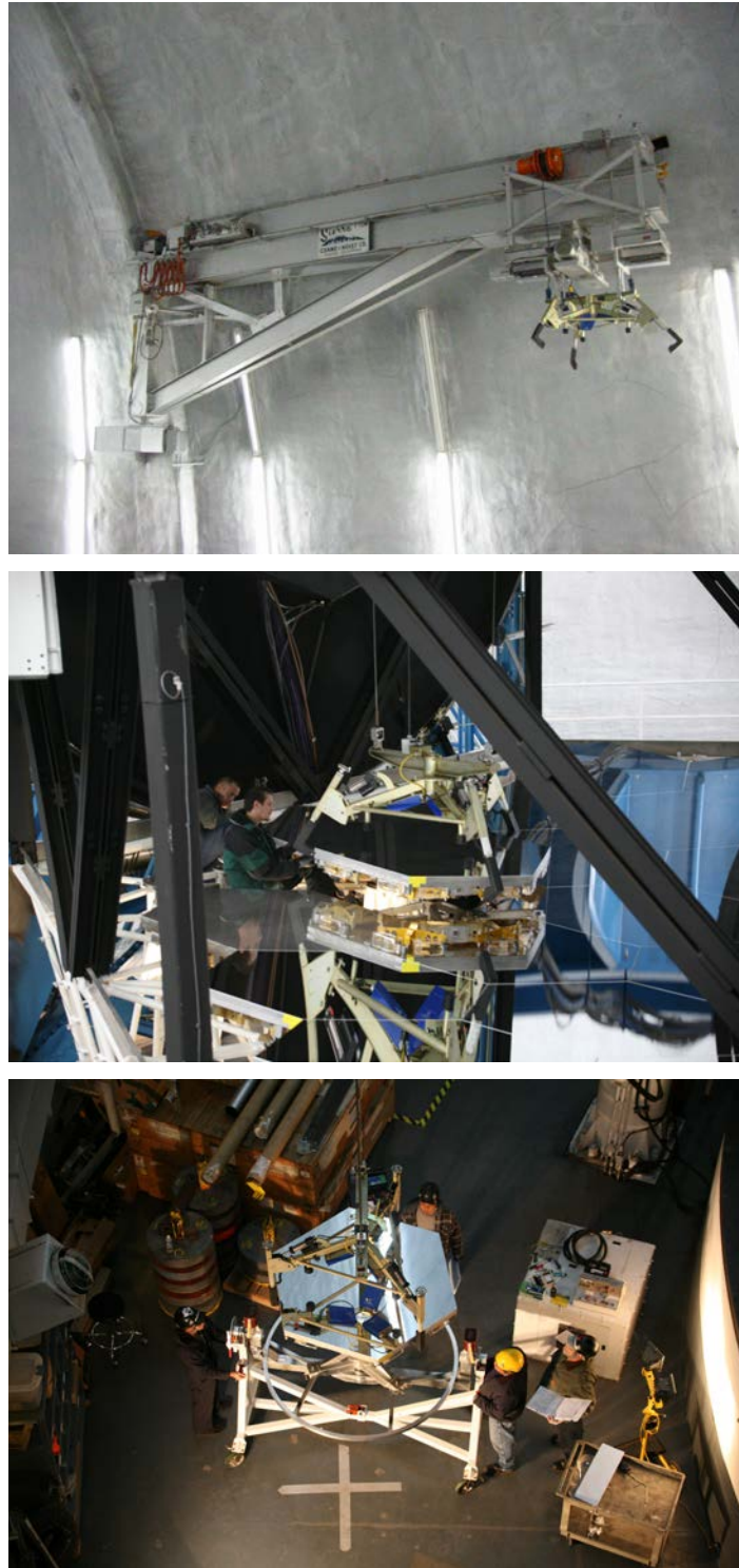
Figure 63: Keck segment-handling system—Enclosure-mounted, segment-handling crane with segment lifting-fixture (top), segment secured on lifting fixture on top of M1 (middle), and segment lowered to handling cart on the observatory floor (bottom).
