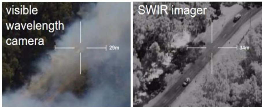
Figure 3.3. SWIR detection enables imaging through smoke and haze. (sensorisinc.com)
