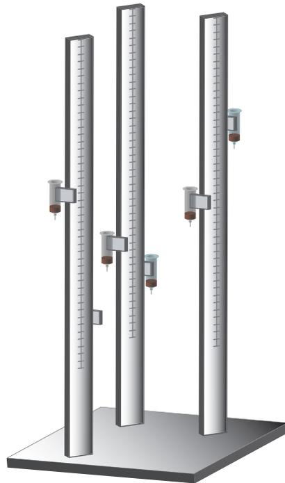
**Figure B.8:** Syringe towers. Made from commercially available erector set, the towers provide support for static syringes. We use a three pillar design with six adjustable platforms, which hold 2-9 syringes each. The ticked lines in the drawing represent rulers that are used for consistent syringe placement. All the parts necessary for constructing the tower are listed in Table B.9.
