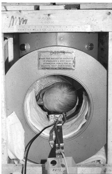
Fig. 5 Brit puts his head in the first one-tesla magnet designed for brain magnetic resonance spectroscopy. Helman's mayonnaise was the "best fit" to Brit's brain.
