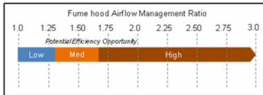
Figure 11. Benchmarks for fume hood airflow management ratio
