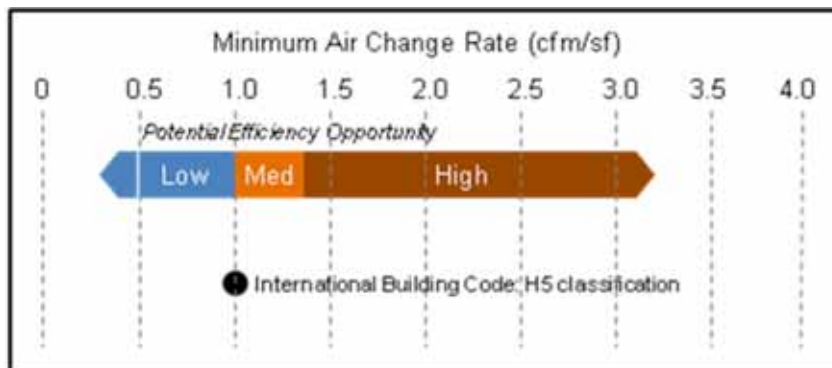
Figure 5. Benchmarks area-based minimum ventilation rates
