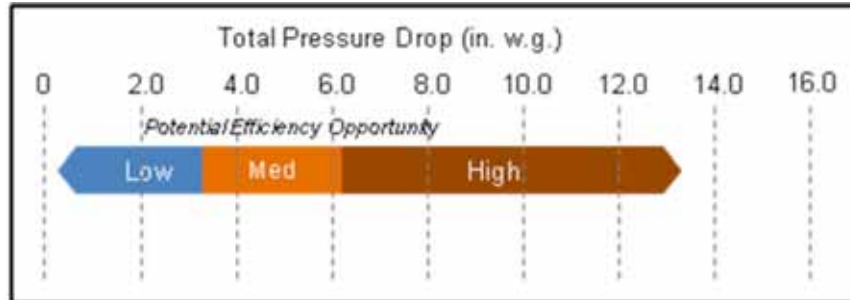
Figure 9. Benchmarks for total system pressure drop.
