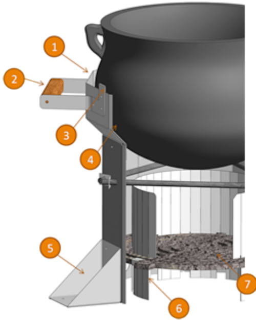
Figure 2: Schematic and picture of the Berkeley-Darfur Stove. The schematic illustrates several design features that are described in the text above.
