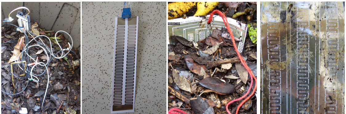
Figure 3.5: The sensing prototype (left), a paper Ag-NP sensor design (c. left, © Adrian Freed 2015), the Ag-NP prototype buried in the compost bin (c. right). Scratches on the sensor's surface proved that the biota's rough texture was not suitable for this design (right).
