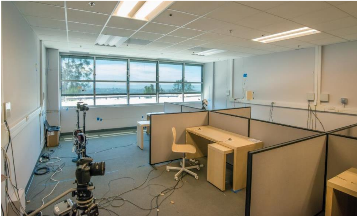
Figure 9. Photograph of the interior of the FLEXLAB testbed office with an exterior roller shade partially lowered over the south-facing window.
