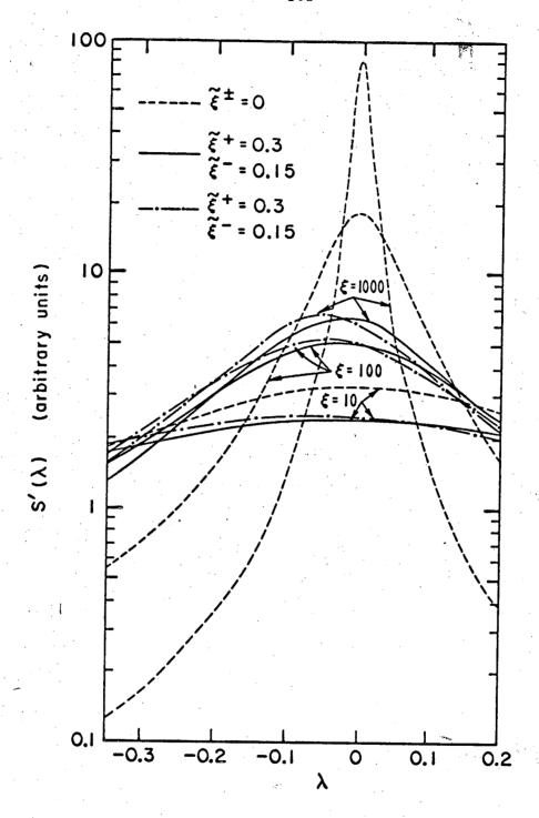
Fig. 22. (See Section VI-F.) The power spectrum vs.  $\lambda$ . The dashed curves are the reproductions of the curves in Fig. 21 for  $\xi$  = 10,100, 1000 for comparison.
