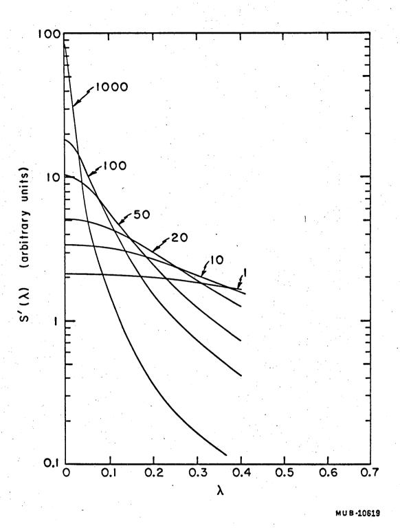
Fig. 21. (See Section VI-F.) The power spectrum  $S'(\lambda)$  vs.  $\lambda$  (see (6-24,29,33) for the definition of the parameters).  $\xi^{+}=0$  for the curves in this figure.  $S'(\lambda)=S'(-\lambda)$ . The numbers labeling the curves are the values of  $\xi$ .
