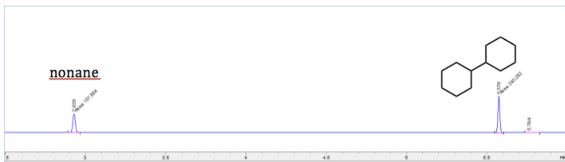
Figure 2.38 GC trace showing one to one mixture of nonane to bicyclohexyl.
