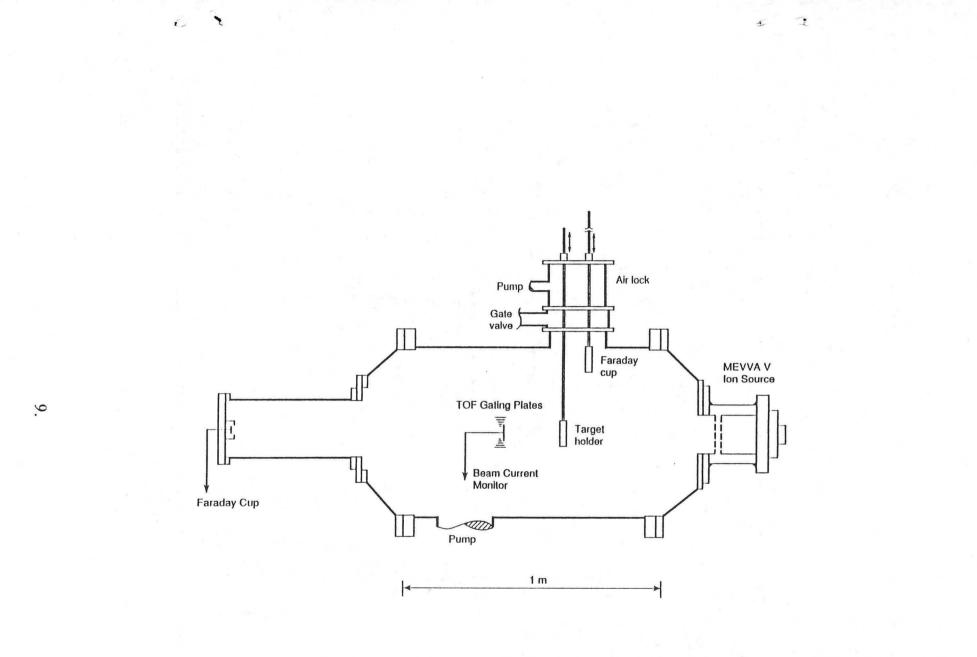
Fig. 2 Schematic of the experimental facility. (XBL 896-7641B)
