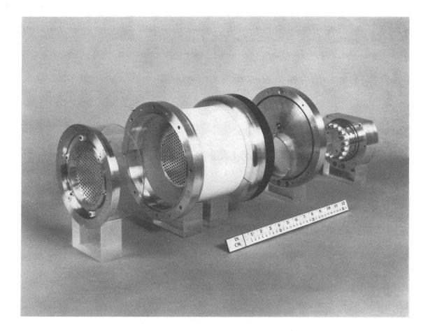
Fig. 1 The MEVVA V ion source, partially disassembled to show the multiple cathode feature (holds 18 separate cathodes) and the large beam formation electrodes. (XBB 892-1124)
